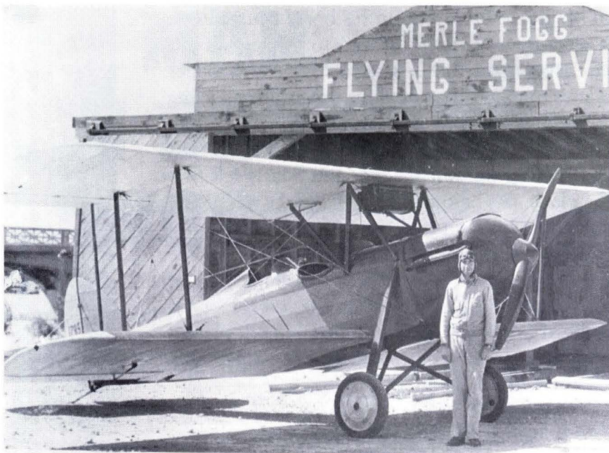
Merle L. Fogg standing by his WACO 10 Biplane. The engine was a 90 horsepower Curtiss 0X5, water-cooled World War I engine that was used in the old Curtiss Jenny plane.
