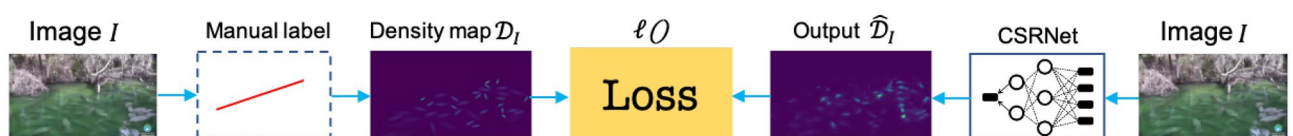
Figure 5. A conceptual view of the deep neural network based manatee counting workflow. From left to middle: An input image ( I ), the line-segment labels of the image, the density map \mathcal{D}_I of the image. From right to middle: An image I is applied to a neural network (NN) to predict its density map \hat{\mathcal{D}}_I . The loss function in the middle is used to regulate and train the NN to ensure that \hat{\mathcal{D}}_I maximally approximates to the ground-truth \mathcal{D}_I .
