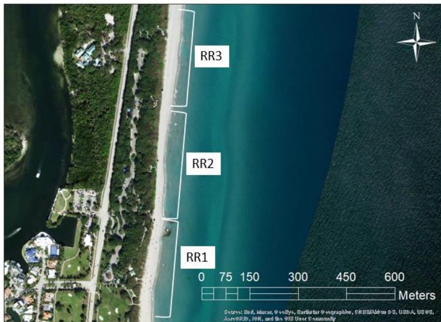
Figure 2. Map of 0.925 km study area that is further sectioned into three 308 m subzones. Within each subzone are survey transects RR1, RR2, and RR3. Transects are the locations of Ground Control Points, RTK survey markers, and sediment collection sites. Nesting data and UAV-derived data are attributed +/- 154 m north and south of each transect.
