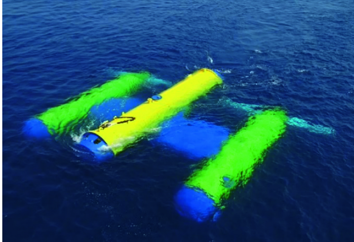
Figure 2.1: Example of a buoyancy-controlled MCT that has counter-rotating rotor blades with a single variable buoyancy module. Image credit IHI Inc. [12, 27].
