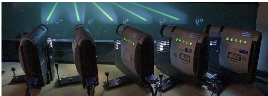
(a) Experimental setup of multiple illumination sources in a large water tank.
