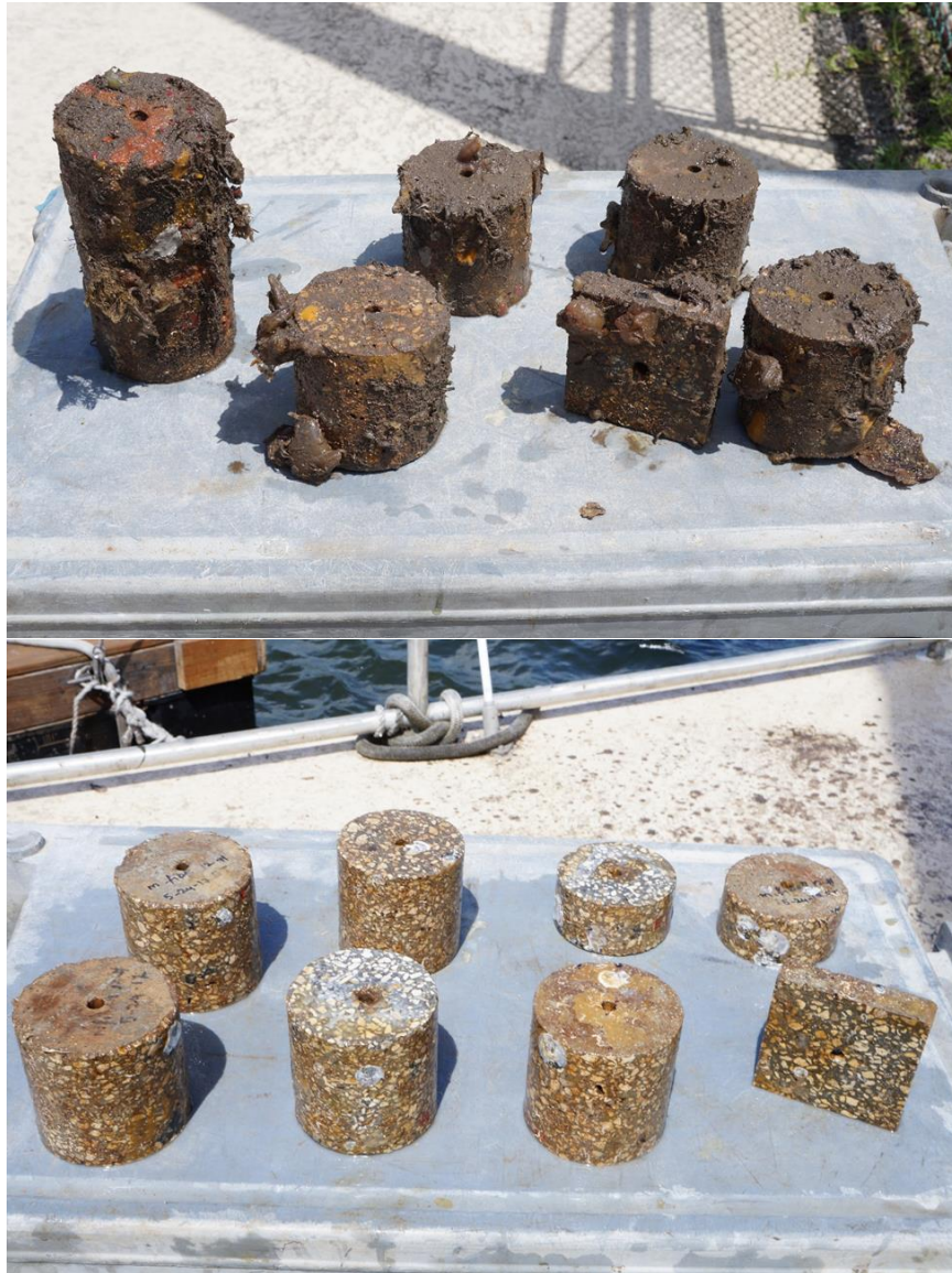
Figure 8-Barge Conditioned Samples Before and After Cleaning.
