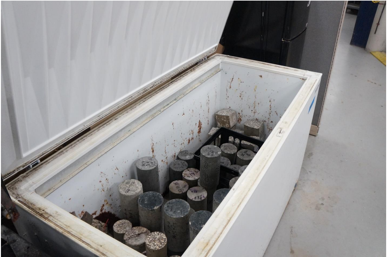
Figure 5-High Humidity Conditioning Chamber.
