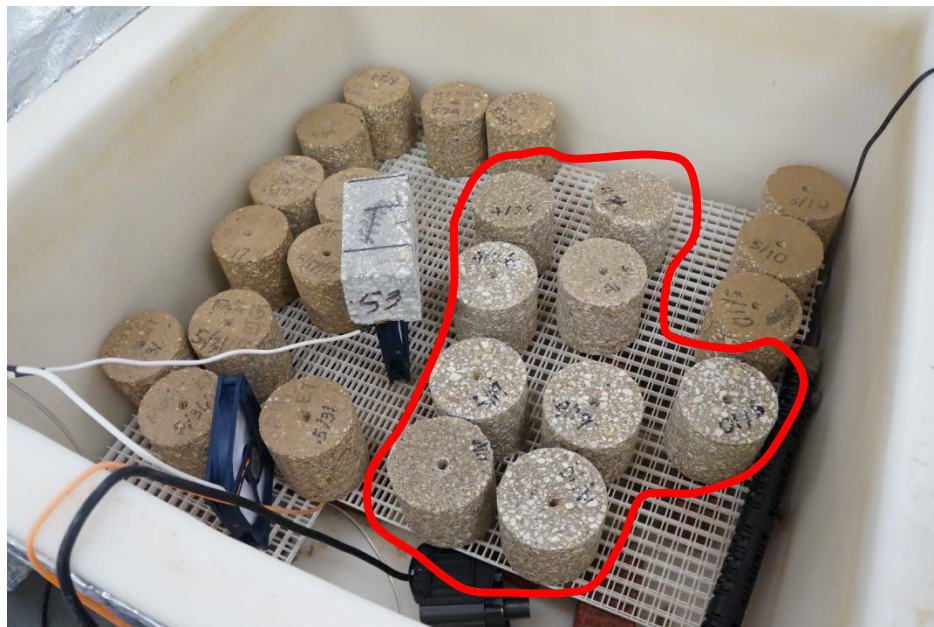
Figure 7-Rinsed High Humidity Cylindrical FRC Samples.
