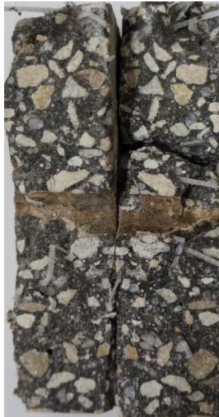
Figure 10-Cross Section of Square Sample's Fracture Plane.
