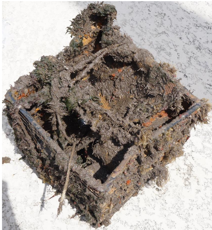
Figure 6-Barge Conditioned FRC Sample Container.
