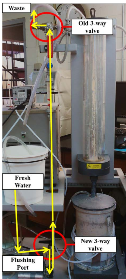
Figure 15: Pump flushing flow path
