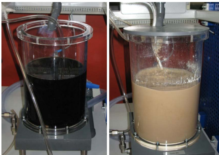
Figure 59: Color comparison for raw leachate (left) vs. leachate w/ \text{TiO}_2 (right)
