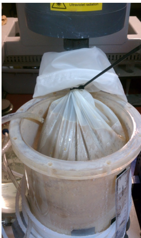
Figure 27: Nylon monofilament filter bag attached to advanced oxidation machine for catalyst recovery
