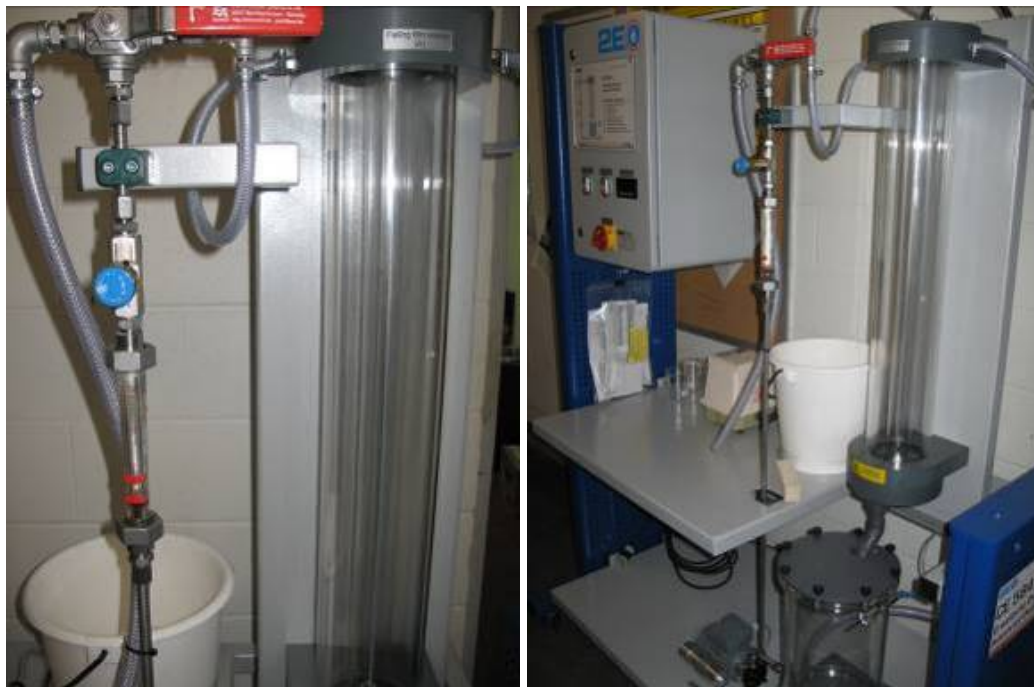
Figure 8: Photographs of the falling film pilot reactor (left: close up view of the reaction chamber; right: overall view).
