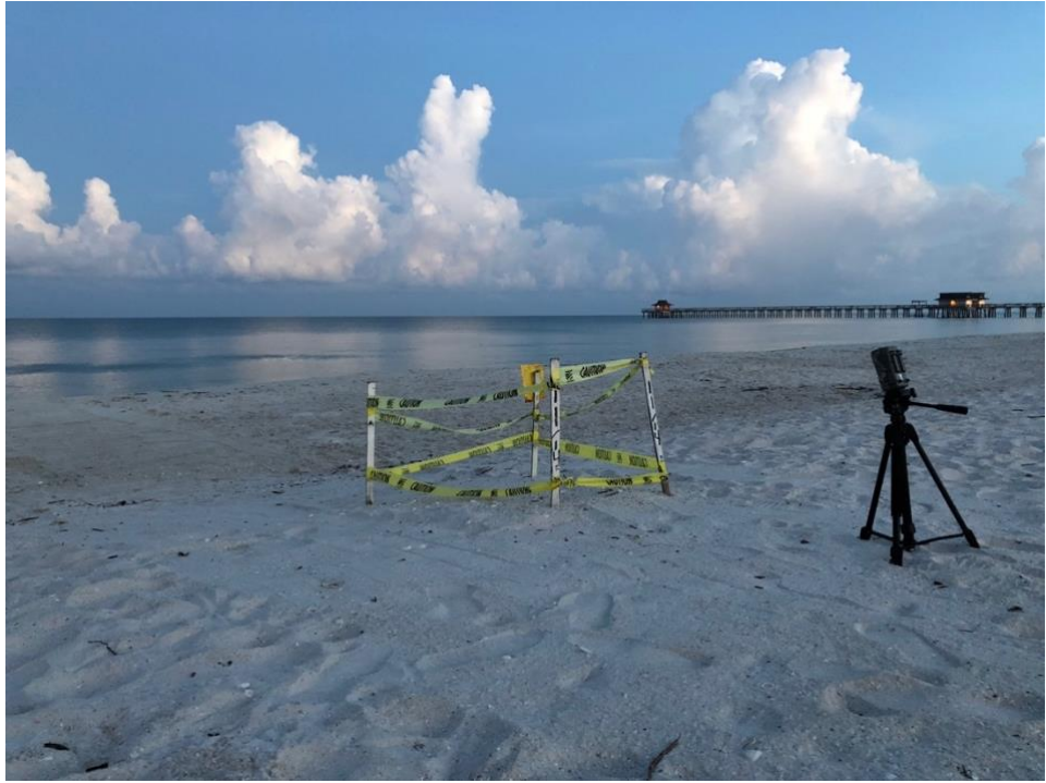
Figure 1. An infrared camera placed behind a nest. Each nest was marked using tape and stakes by local beach surveyors. Photo by B. Villegas Vindiola
