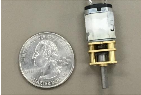
Fig. 16. Geared DC motor selected next to quarter
