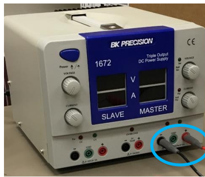
Fig. 19. BK Precision 1672 variable power supply utilizing one power and one ground connection
