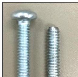
Fig. 40. Original versus cut and sanded screw
