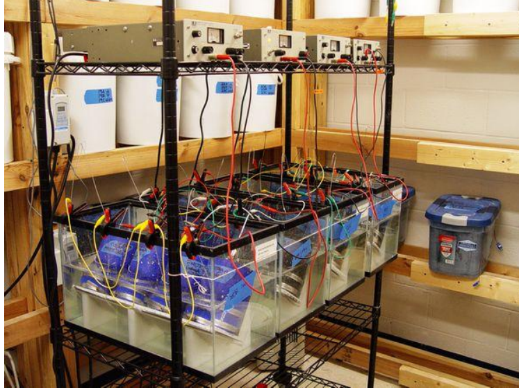
Figure 6.2: Schematic illustration of setup for RCM test at 30 °C and 40 °C.
