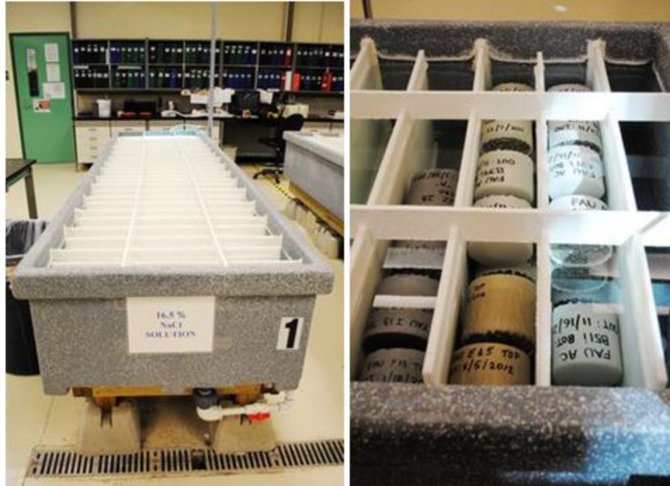
Figure 4.3: Exposure tank for bulk diffusion test in FDOT.
