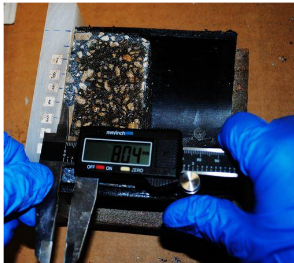
Figure 5.4: Measurement of chloride ion penetration depth.
