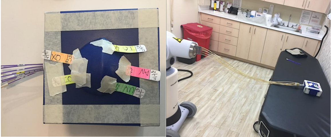
Figure 23: Left) Phantom with the SAVI and TLDs in place. Right) Phantom connected to the afterloader, ready to be irradiated.
