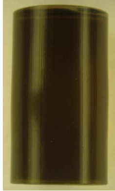
Figure 5.20: Failed VE 510A compression specimen ( 85% RH at 50°C).
