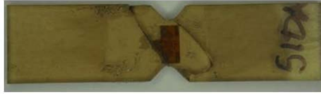
Figure 5.23: Failed VE 510A Iosipescu shear specimen.
