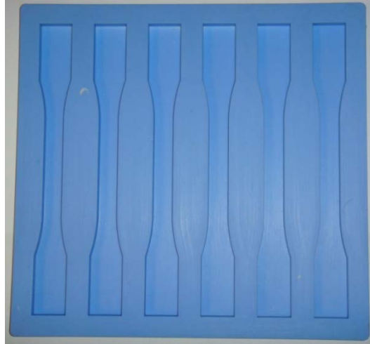
Figure 4.3: Open face silicon mold for dog-bone tensile test specimens.
