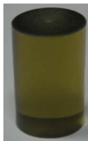
Figure 4.10: Neat resin compression specimen.
