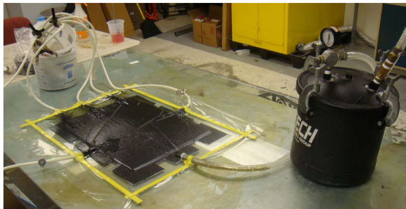
Figure 4.13: VARTM manufacturing configuration.
