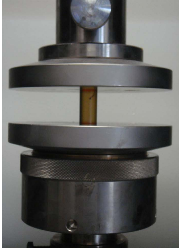
Figure 4.18: Neat resin compression test set-up.
