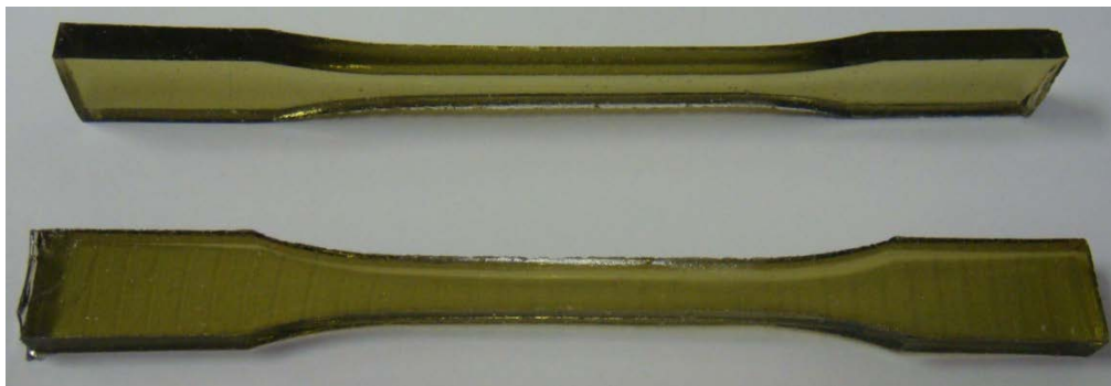
Figure 4.4: Tensile specimens from an open faced mold.
