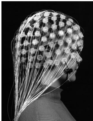
Figure 1.1. A geodesic net with 128 electrodes from [47].
