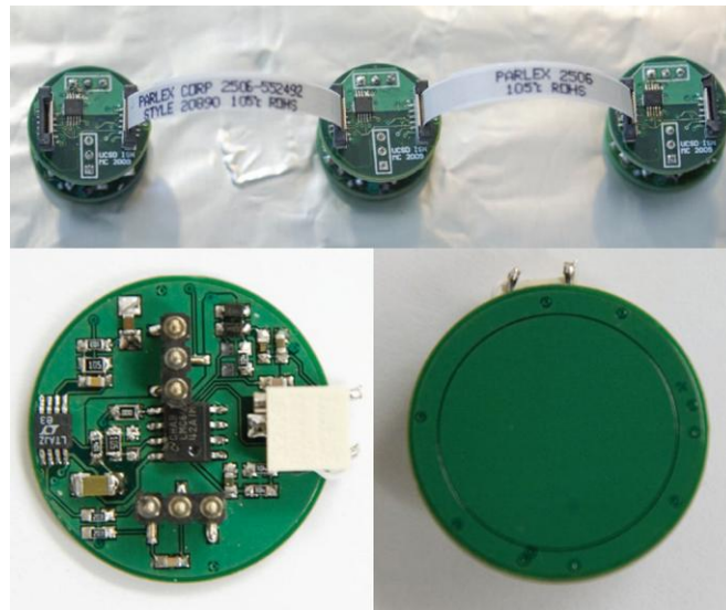
Figure 2.11. Micropower active non-contact EEG electrode from [17].
