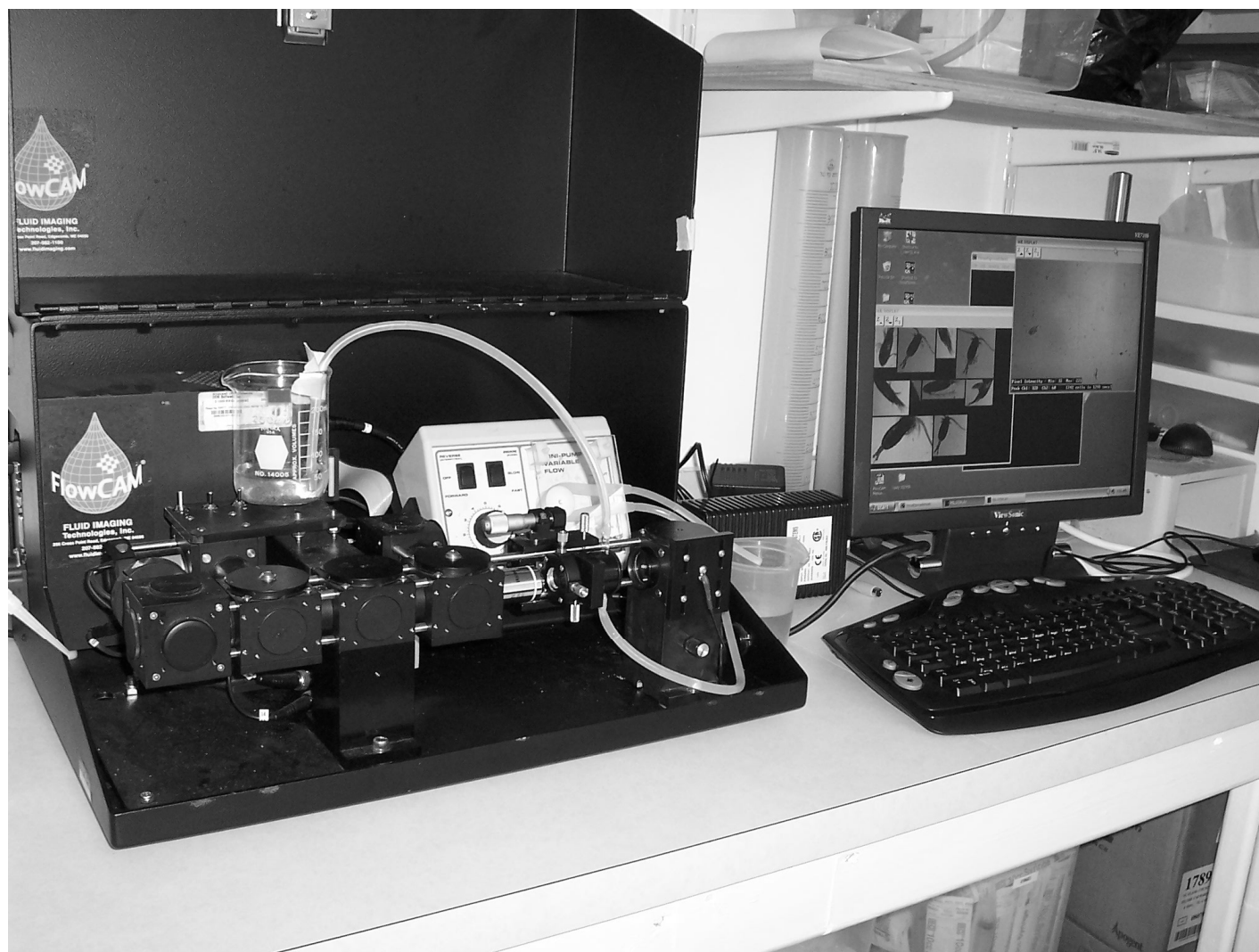
Figure 2. FlowCAM set-up with sample running and images being collected on the computer.
