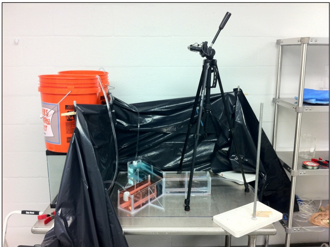
Figure 6. Experimental setup with sources for A and B flowing in from the orange buckets, through the tank, and out the overflow tube. Dye shows separation of chemical cues until reaching Region C. Camera mounted on tripod over Y-maze to record trials and black plastic eliminates visual cues.
