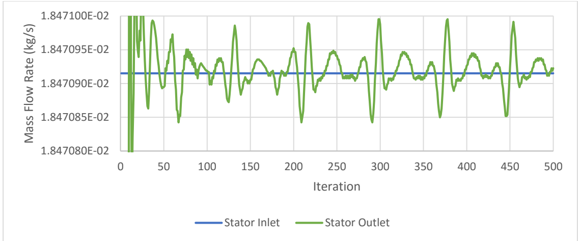
Figure 32: Mass flow rate surface monitor at stator planes ( SST – Transition – CC, M5 )
