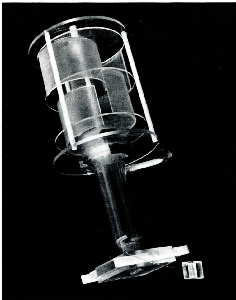
FIG. 2. In situ incubation chamber used to determine seagrass productivity.
