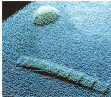
Fig 4: 400 x 400 pixel range maps of dome and step wedge test objects recorded in clear water at a nominal range of 1 metre (NCEL).
