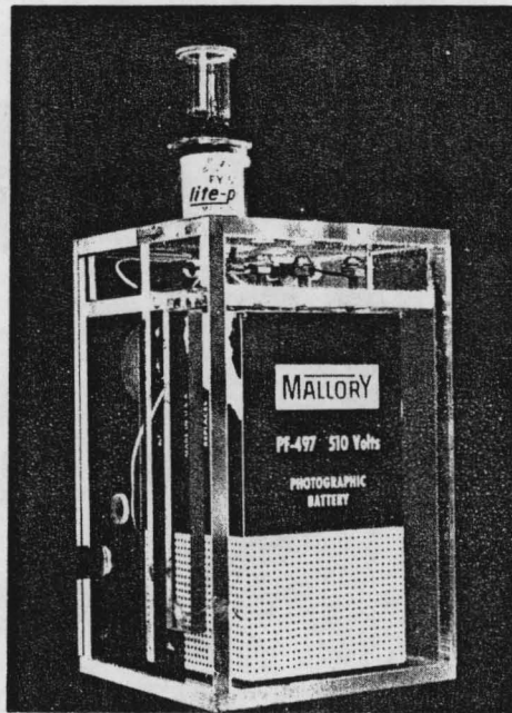
Figure 8. Assembled DC powered FX-265 flash unit.
