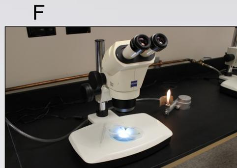
(Picture F) Dissecting Microscope with a gas burner, Petri dishes, and a worm pick
