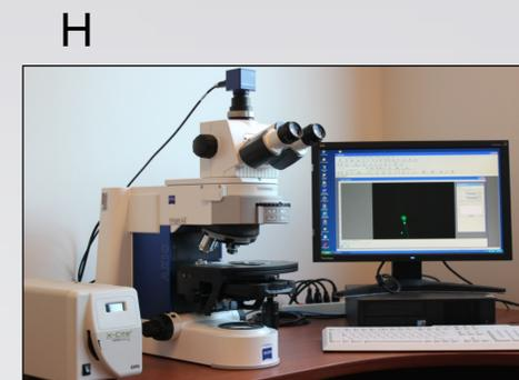
(Picture H) Fluorescence Microscope with an Imaging System
