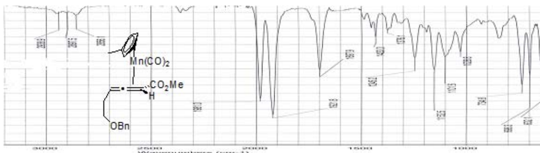
Figure 16. IR spectrum of manganese-coordinated allenyl ester.
