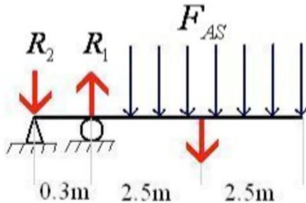
**Figure 3-2 Solid Mechanics - Aerodynamic Reaction Forces**
