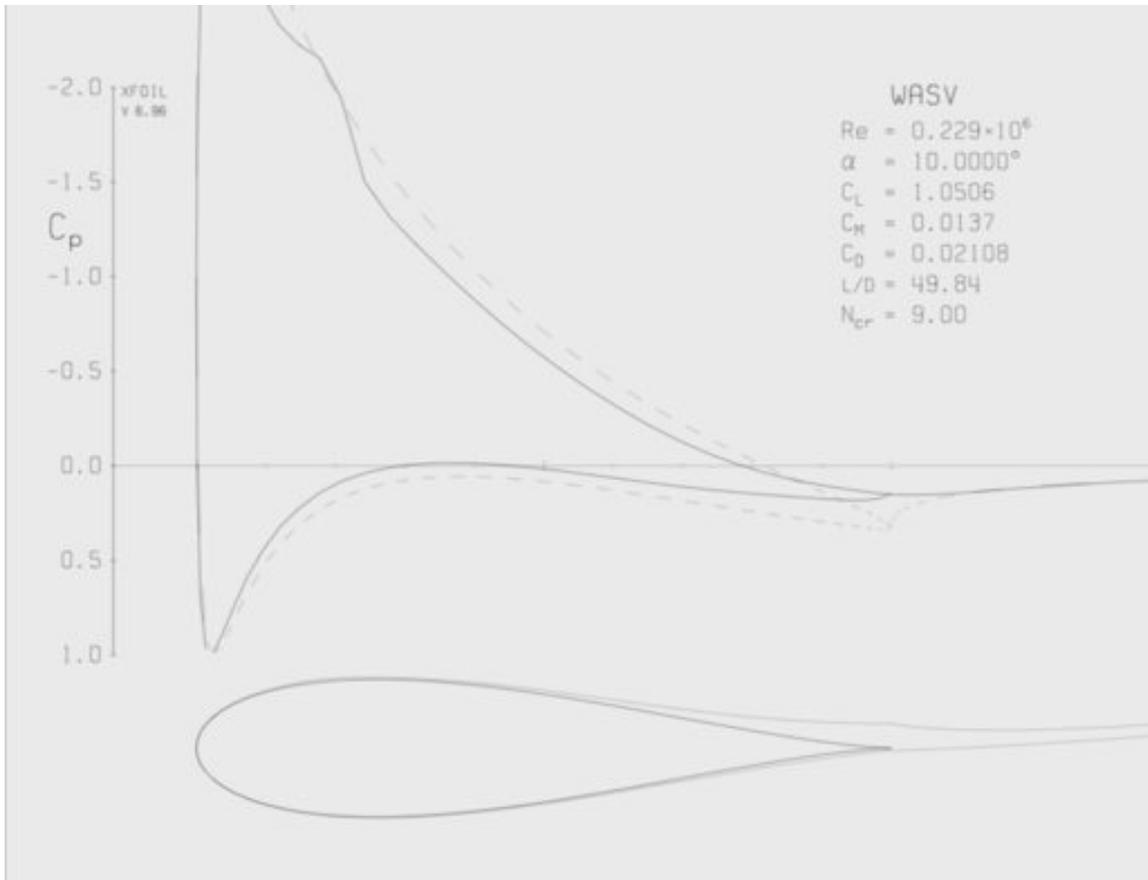
**Figure 2-11 WASV Wing Polar Plot (XFOIL)**
