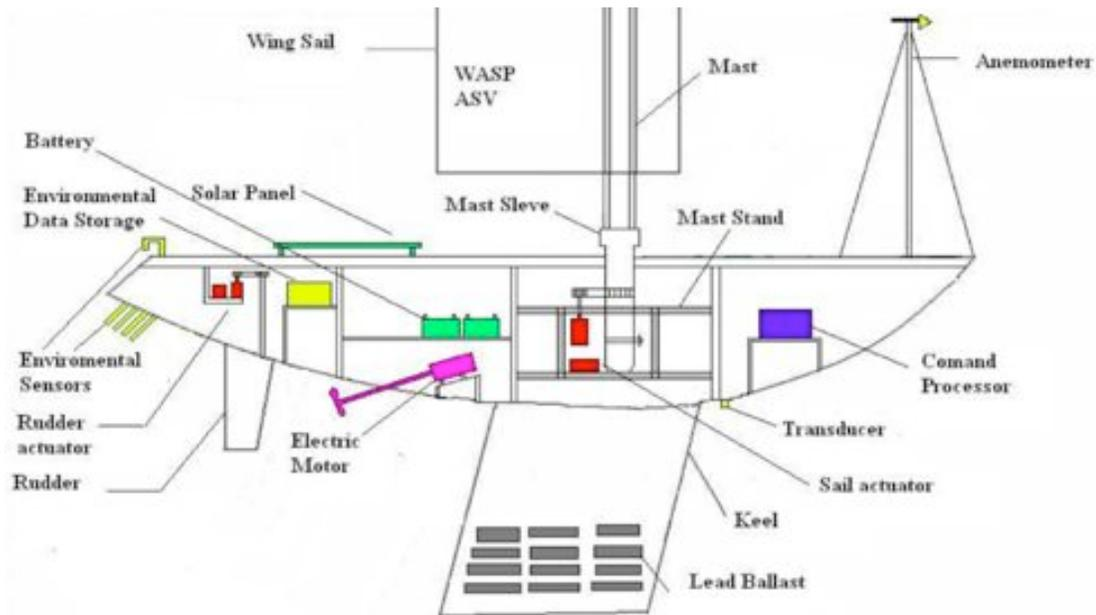
**Figure 1-9 WASP System Diagram [21]**
