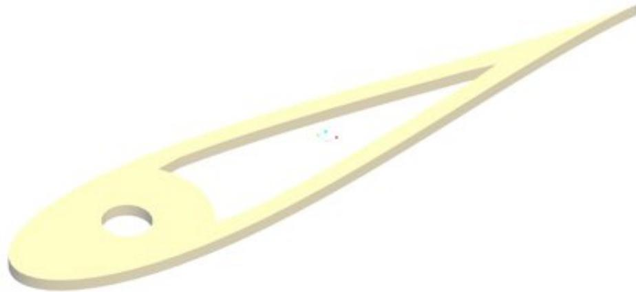
**Figure 3-5 C.A.D Representation of Master Rib**
