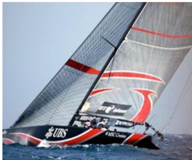
**Figure 2-3 A monohull keelboat is self-righting and modern designs have broadened the speed range beyond Froude numbers of 0.45 [13]**
