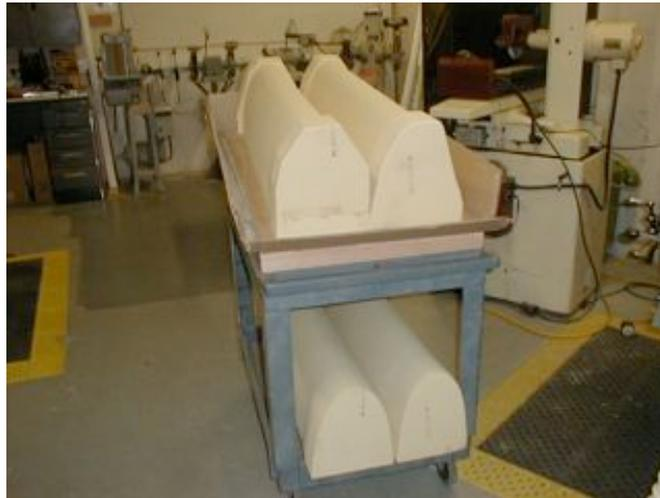
**Figure 7-3 Plug Sections ready for alignment**
