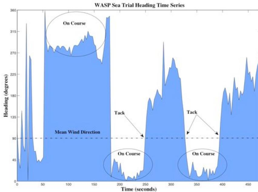
**Figure 5-2 09/12/08 Sea Trial Heading Time Series**
