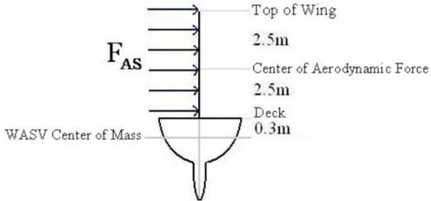
**Figure 3-1 Front View Aerodynamic Heeling Moment**
