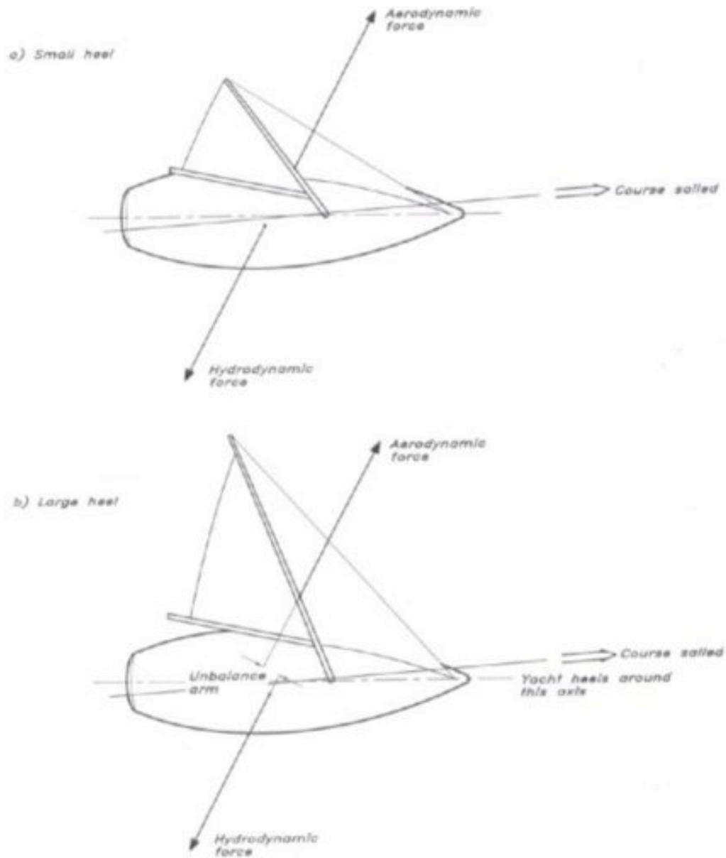
**Figure 2-7 The effect of large roll angles on lead. [15]**
