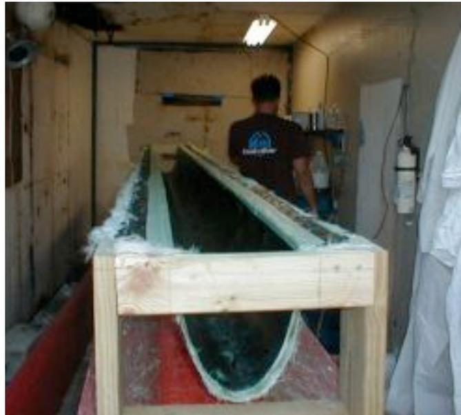
**Figure 7-6 Final female mold**
