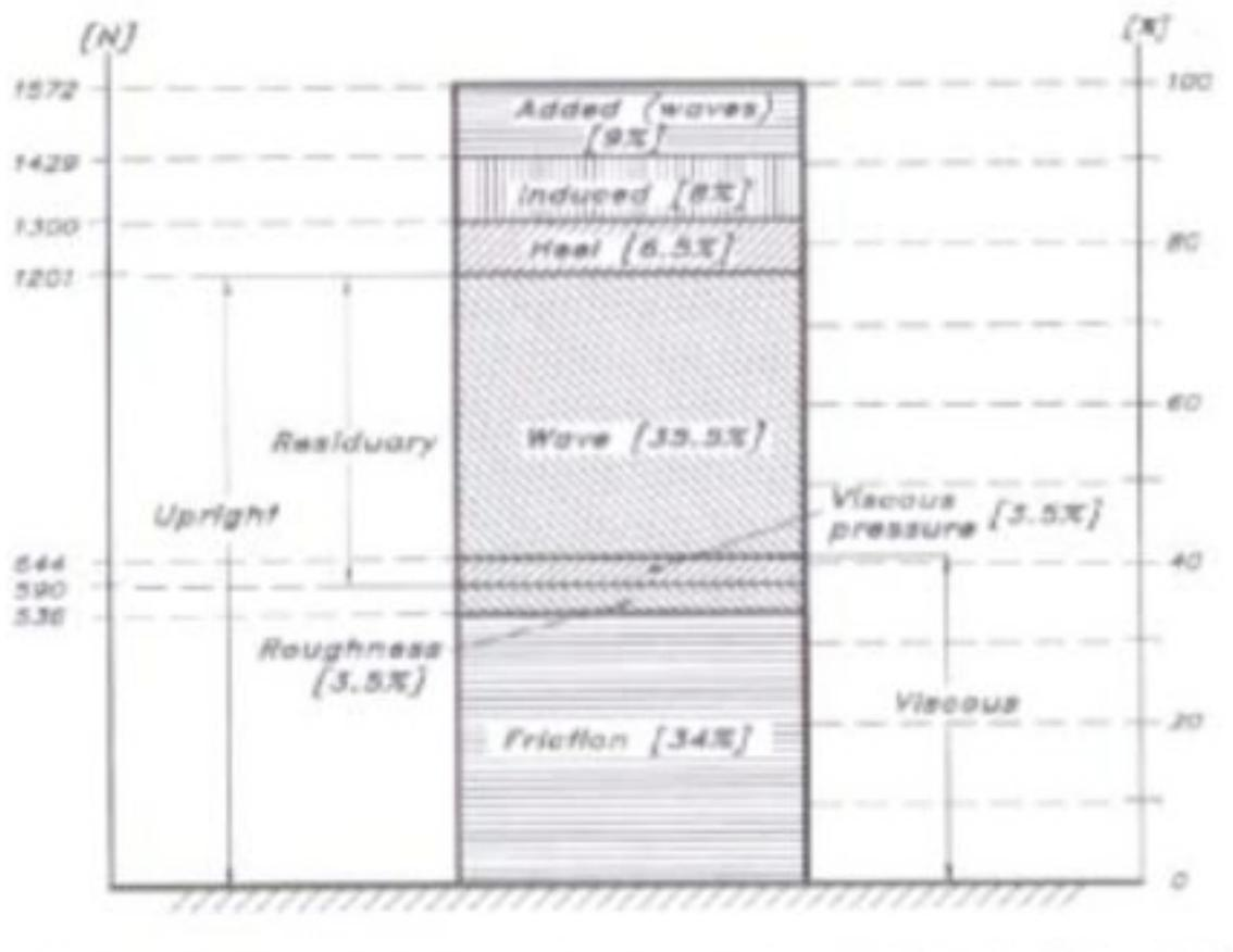
Figure 4-2 YD-40 Resistance Breakdown [15]
