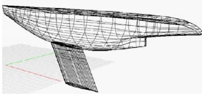
**Figure 2-5 C.A.D representation of 2.4 Meter Hull**
