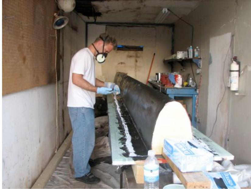
**Figure 7-5 Applying fiberglass and resin to plug**
