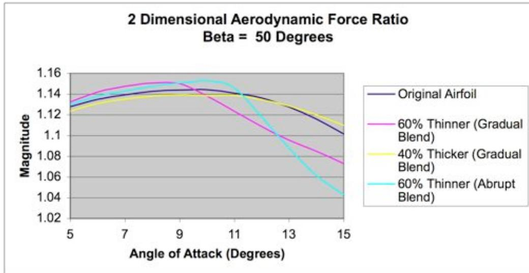
**Figure 2-14  $F_{AR} / F_{AS}$  Variation Plot - The effect of leading edge modification on airfoil performance in two-dimensional viscous flow. Note that the position and magnitude of the maximum thickness of each airfoil is the same.**
