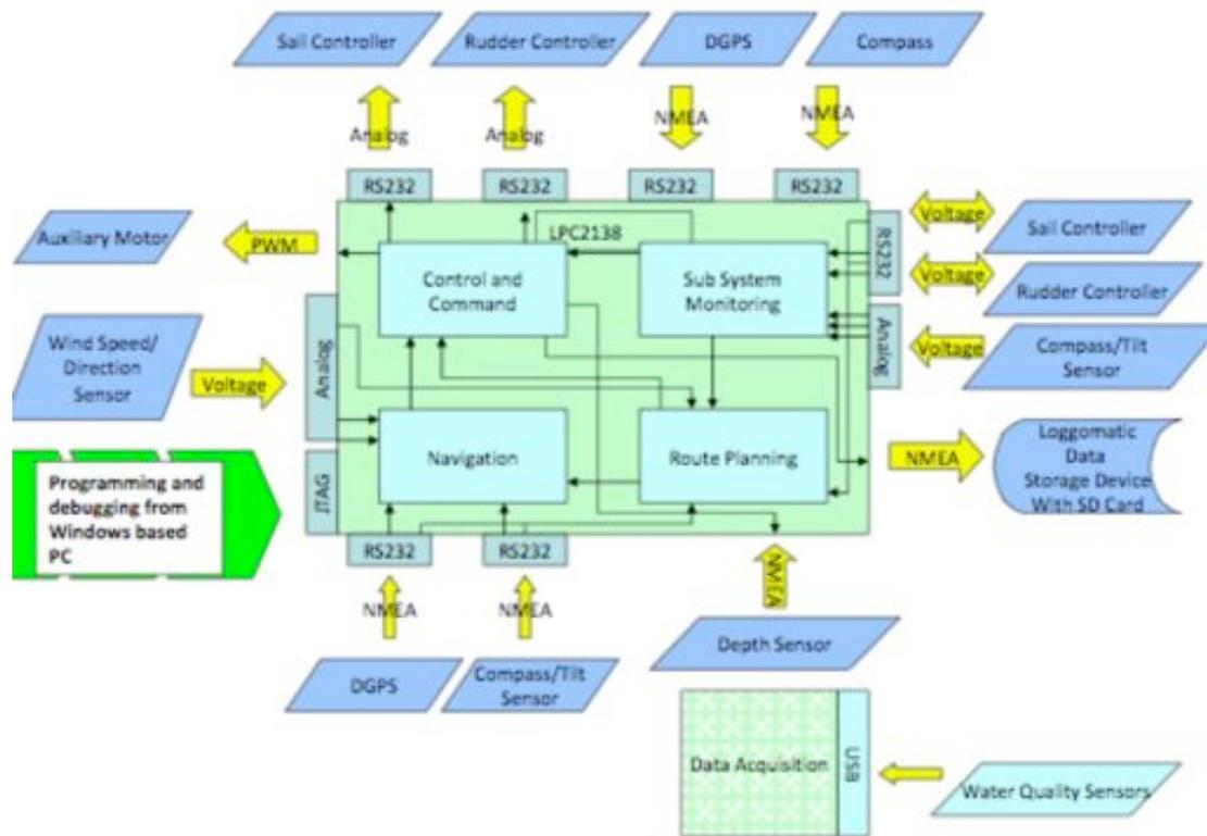
Figure 4-11 Functional block diagram of command & control system [19]
