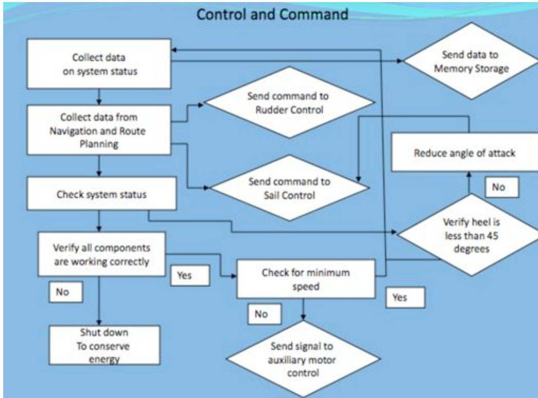
**Figure 4-10 Command & Control Structure [19]**
