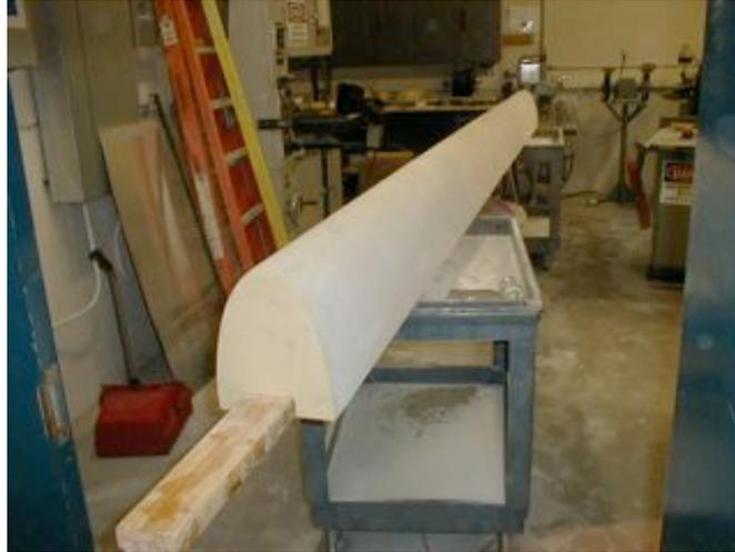
**Figure 7-4 Aligned plug sections after sanding**
