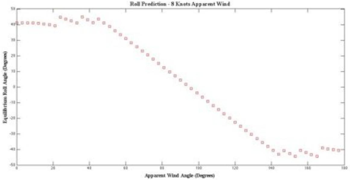
**Figure 4-4 Initial Roll Angle Prediction 8 Knots**
