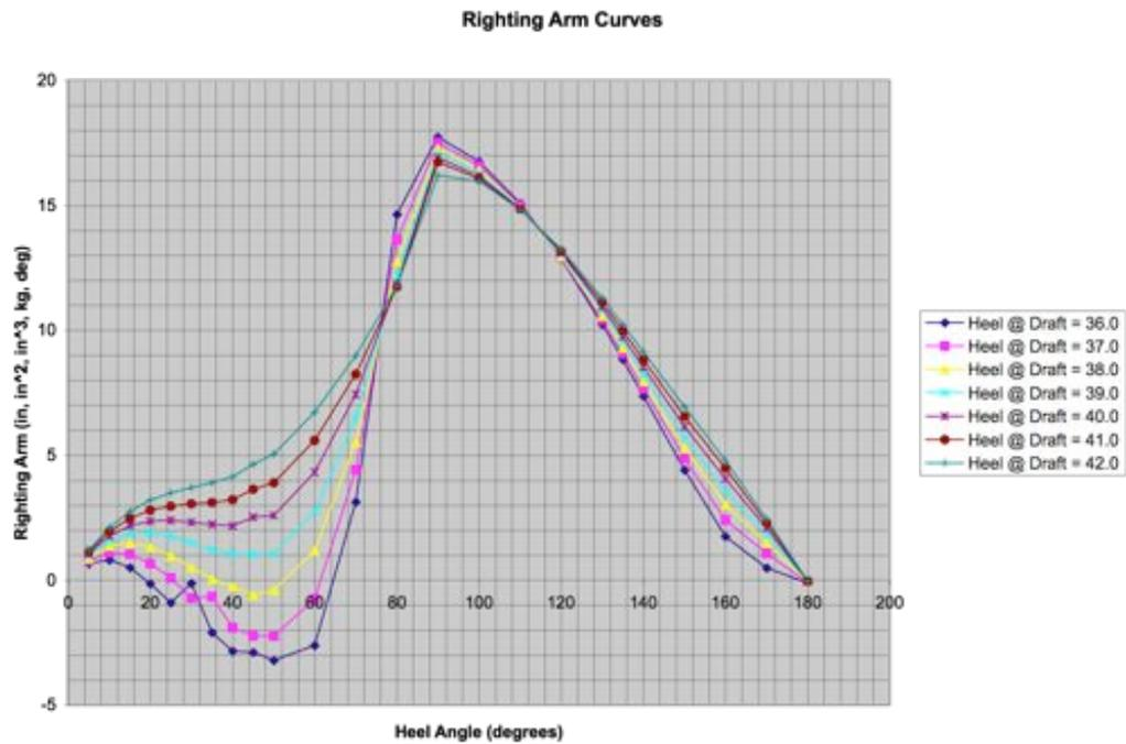
**Figure 2-6 The roll stability plot suggests a region of equilibrium around 45 degrees. The plot also shows that increased loading (correlating to a deeper draft) increases the overall stability in roll.**
