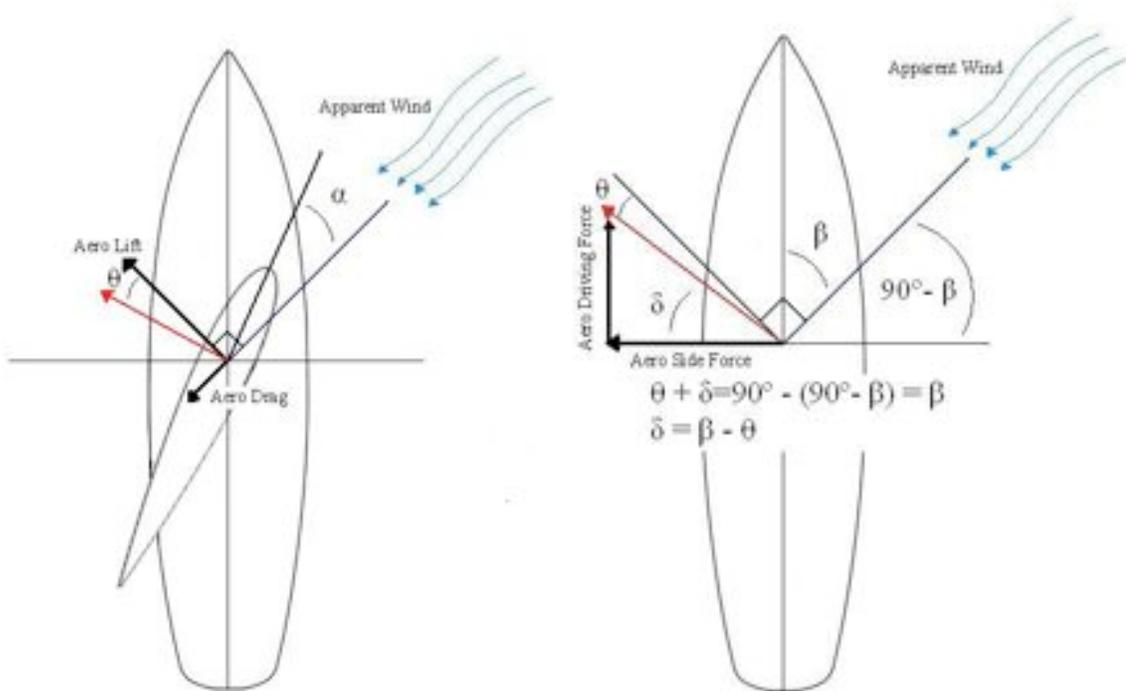
**Figure 2-10 Sailboat Aerodynamic Free Body Diagram**
