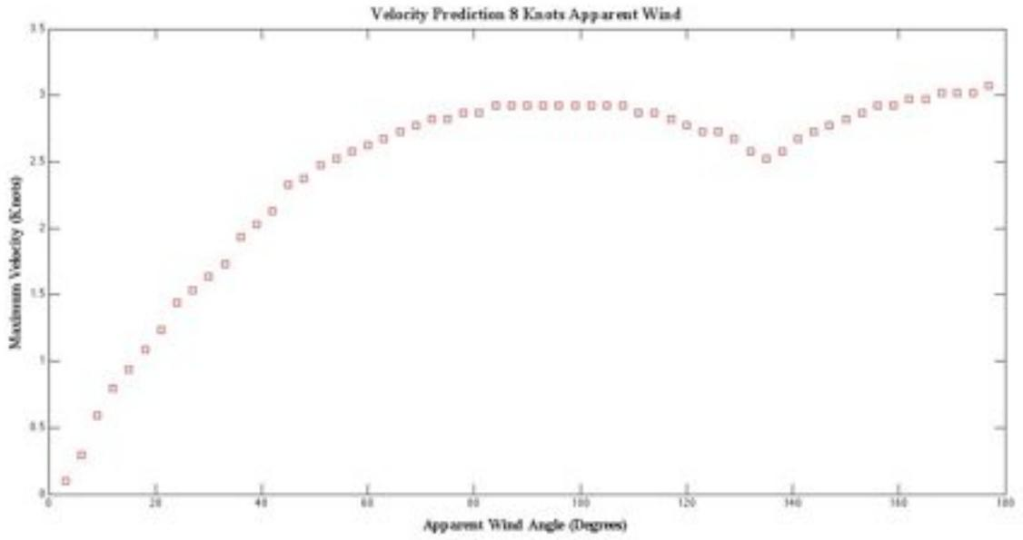
**Figure 4-7 Final Velocity Prediction 8 Knots**
