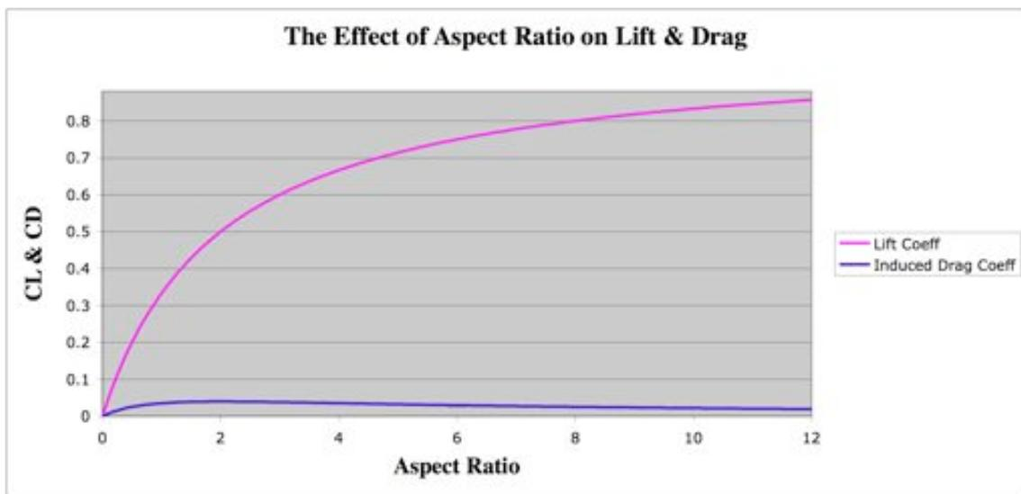
**Figure 2-13 Effect of Aspect Ratio**
