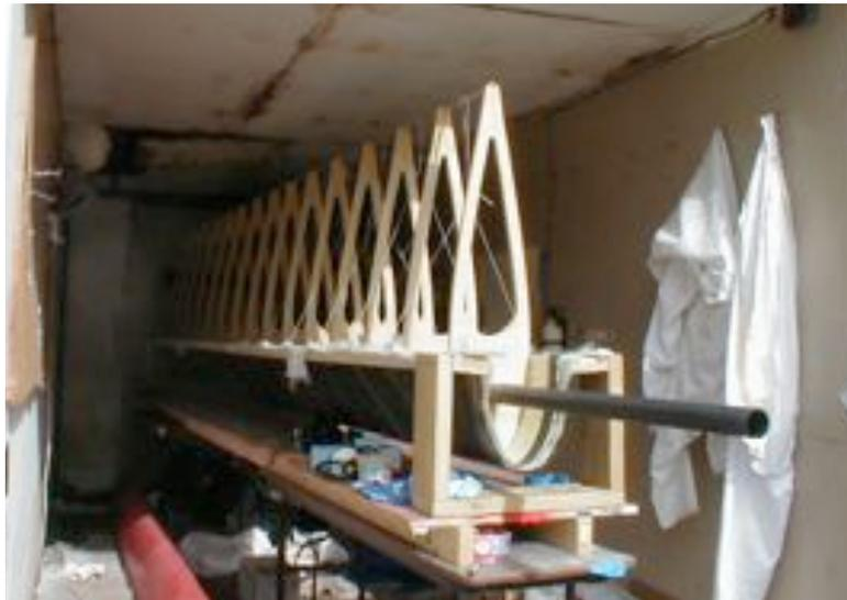
**Figure 7-9 Skeleton & Shell curing**
