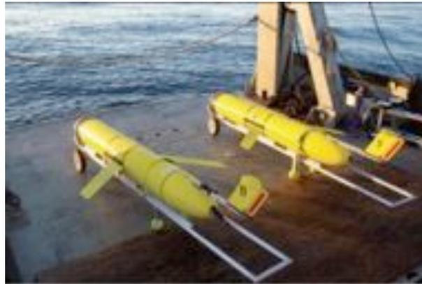
**Figure 1-1 Slocum Glider AUV [3]**
