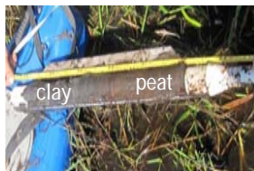
Figure 3. Image of core showing interface between peat and clay
