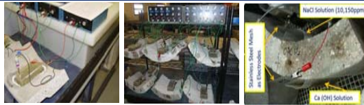
Figure 1 Potentiostatic Figure 2 Galvanostatic Figure 3 Migration Figures 1 – 3 show the three different accelerated transport methods used. The chloride concentration used is within the range found in the field.
