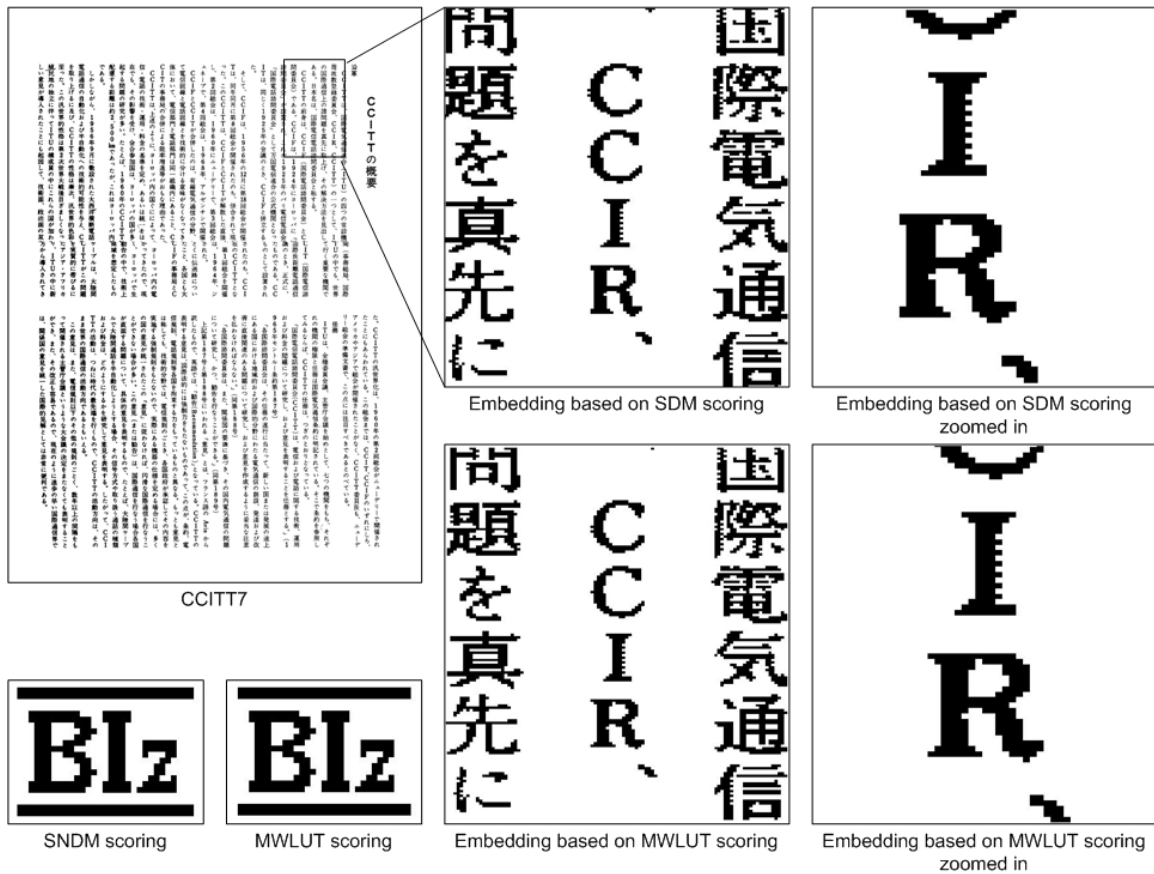
Figure 8 confirms that embedding based on the SNDM pixel scoring results in watermarked images with less visible distortion than embedding based on the MWLUT scores. The Biz logo message is embedded as a robust watermark into the CCITT7 document image using uniform quantization with step size Q=22 . Visual inspection of the zoomed in portion of the watermarked document image reveals that various artifacts are more visible when watermark is embedded using pixel candidates selected according to their MWLUT scores. This visual inspection of watermarked images supports DRDM visible distortion results presented in Table 3.
