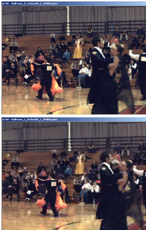
Figure 2. Stereo views with asymmetric view quality. Top: right view coded at 6 Mbps (39.6 dB PSNR); Bottom: left view coded at 1 Mbps (30 dB PSNR).
