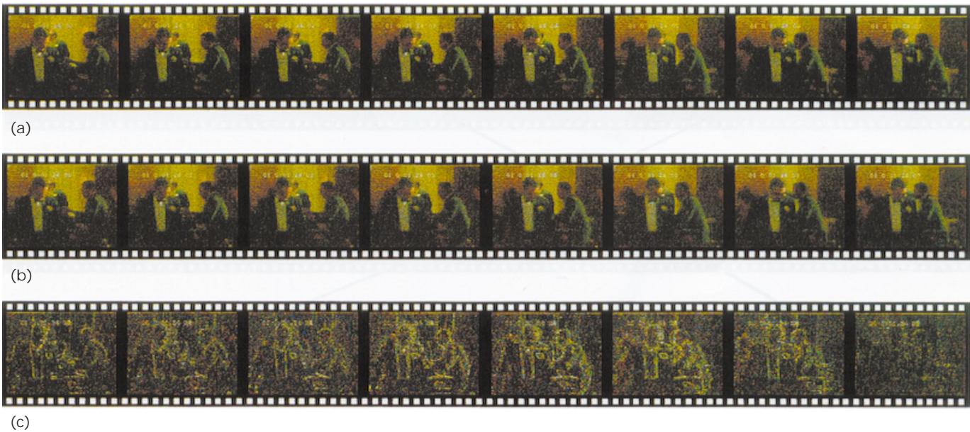
Figure 3. Demonstration of the XYZ video compression technique using eight frames from the movie “Dick Tracy.” (a) Original sequence, (b) decompressed sequence (compression ratio = 101.7, RMS = 0.120), and (c) error between frames multiplied by 16.
