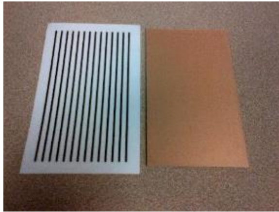
Figure 9 Circuit board and straight decal patterns
