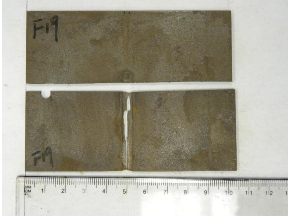
Figure 43 Photo of fractured sample F19 (90%)
