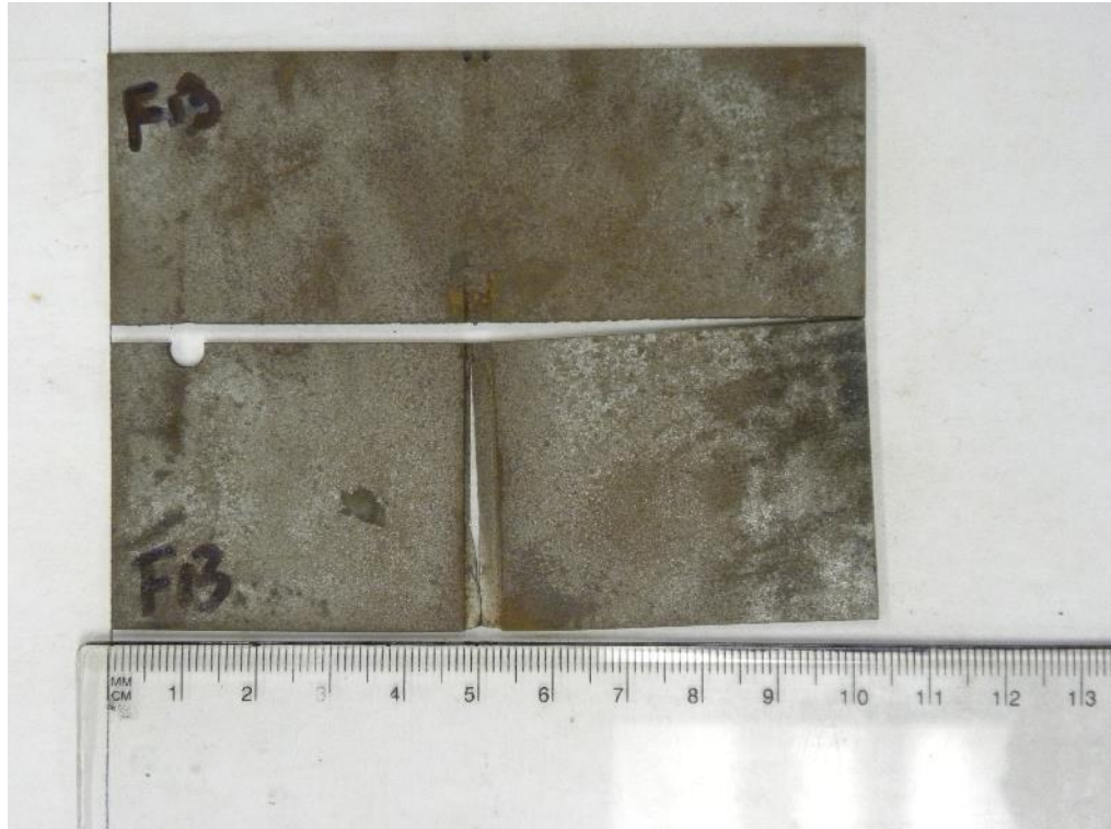
Figure 61 Photo of fractured sample F13 (70%)
