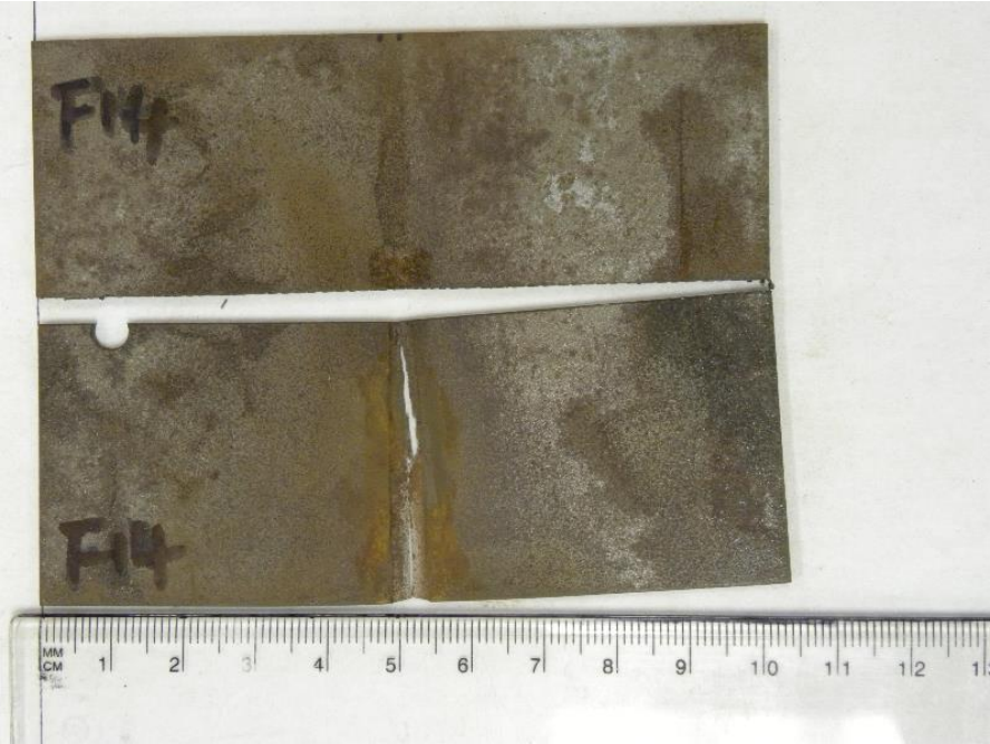
Figure 64 Photo of fractured sample F14 (70%)
