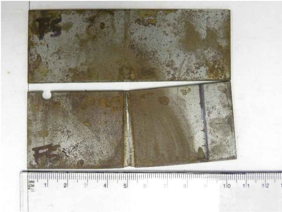
Figure 46 Photo of fractured sample F5 (80%)
