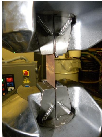
Figure 32 Sample gripped for fatigue testing
