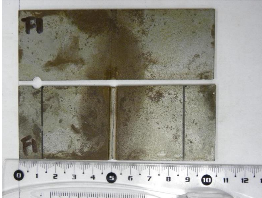
Figure 35 Photo of fractured sample F1 (90%)
