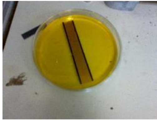
Figure 10 Small piece of circuit board with decal patterns on in etching solution
