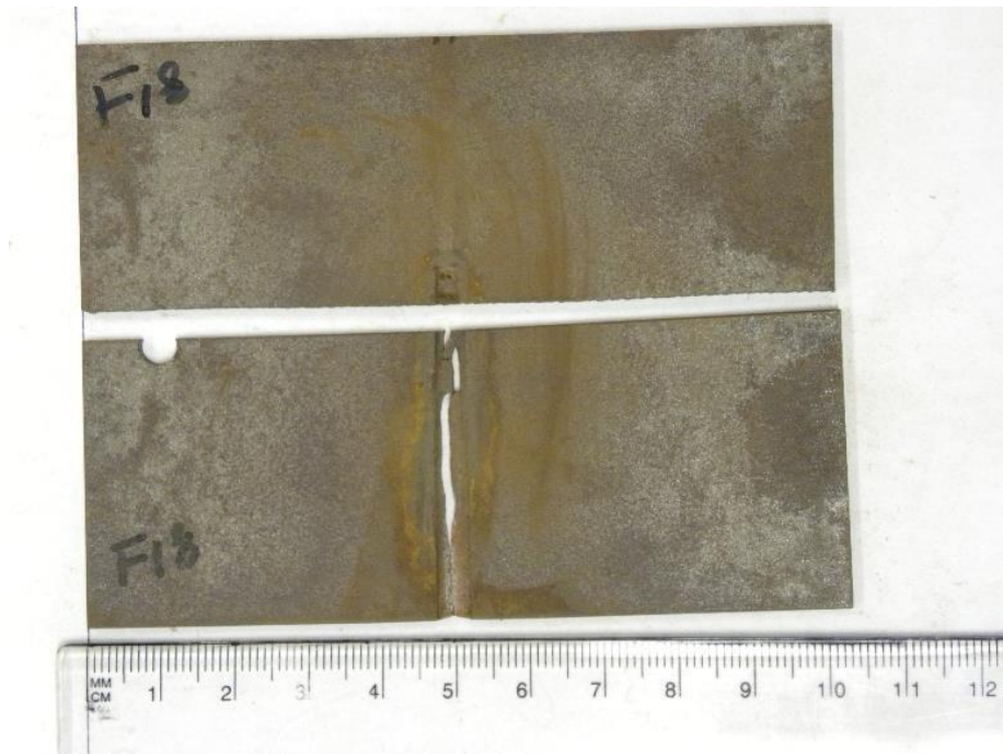
Figure 73 Photo of fractured sample F18 (60%)
