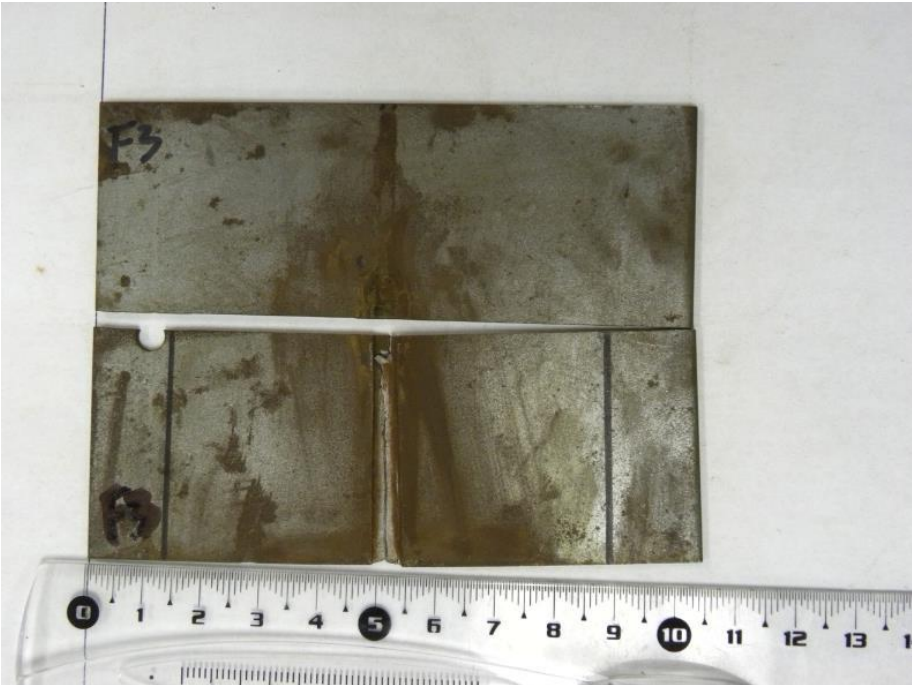
Figure 40 Photo of fractured sample F3 (90%)
