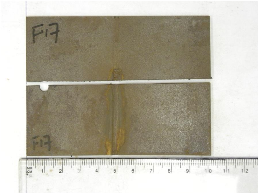
Figure 78 Photo of fractured sample F17 (50%)
