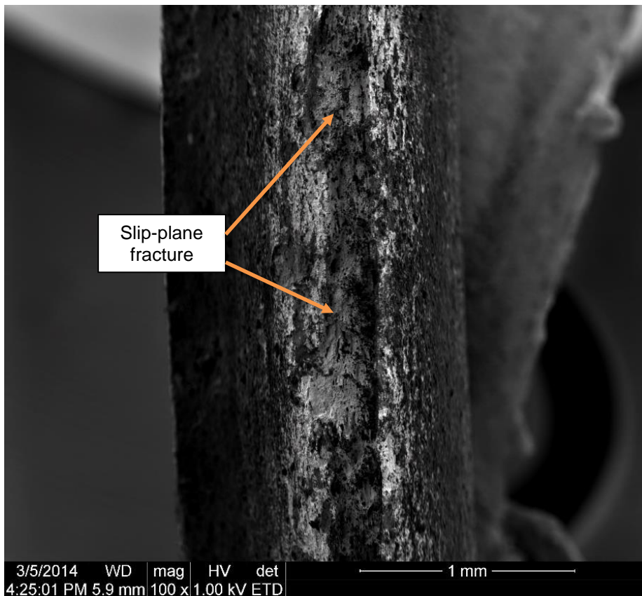
Figure 83 SEM fractograph at location b) of F6. 100 X.
