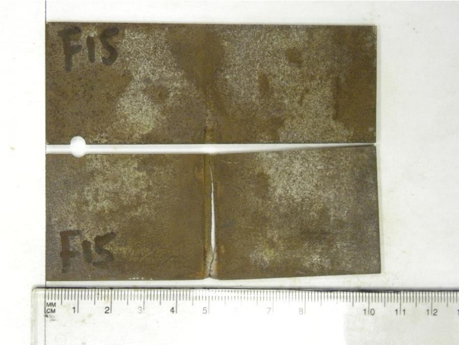
Figure 70 Photo of fractured sample F15 (60%)
