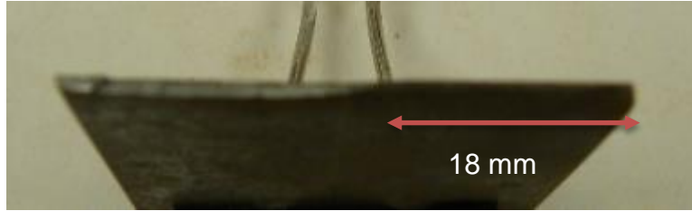
Figure 65 Photo of fracture surface of sample F14 (70%)
