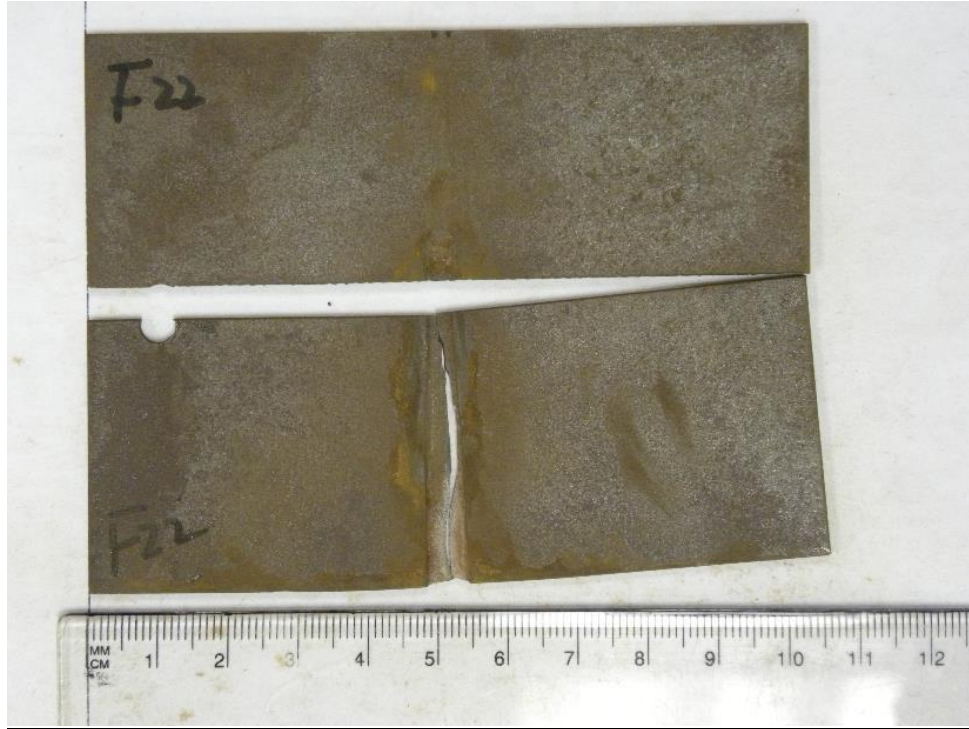
Figure 67 Photo of fractured sample F22 (70%)
