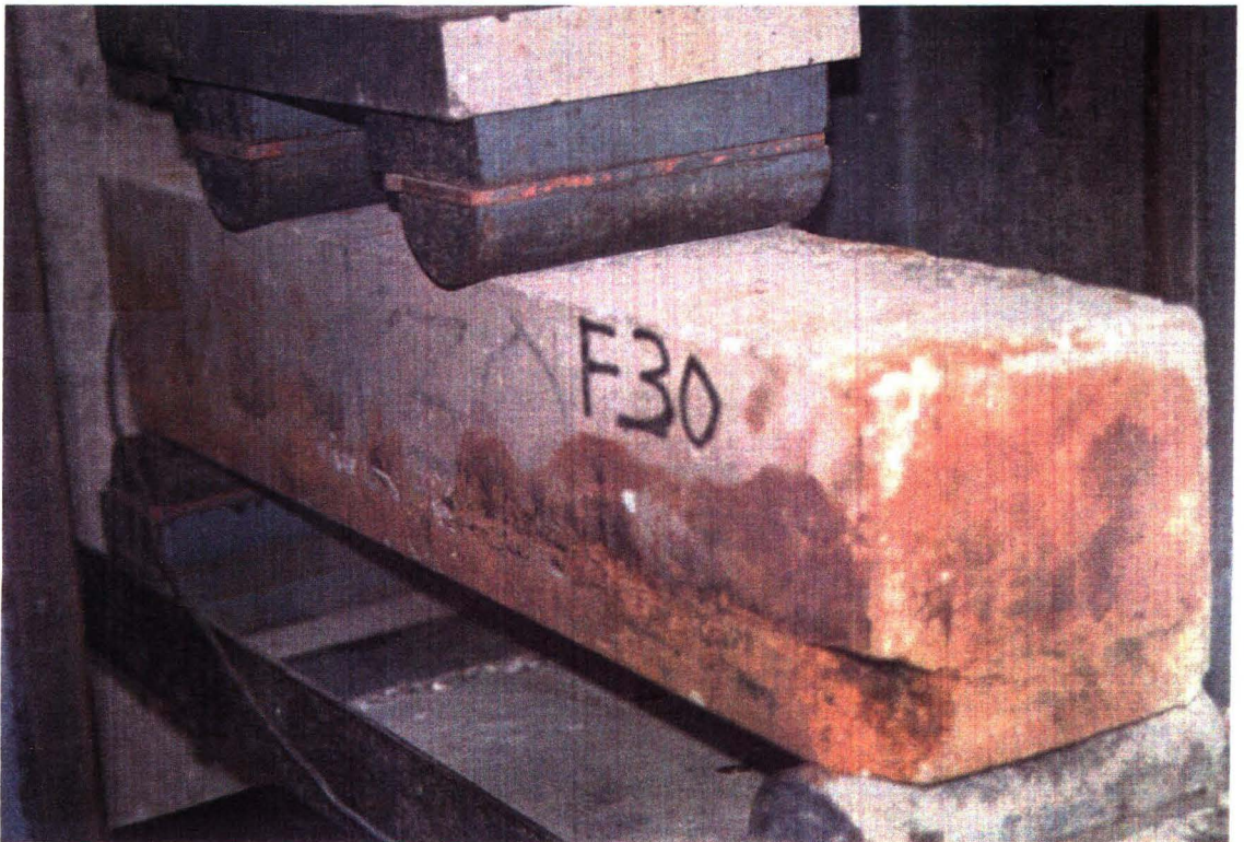
Fig. 5.20 Photographs of flexure test setup.
