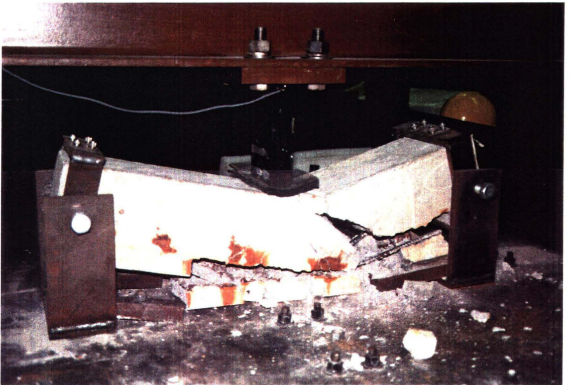
Fig. 5.23 Photographs of the impact test setup.
