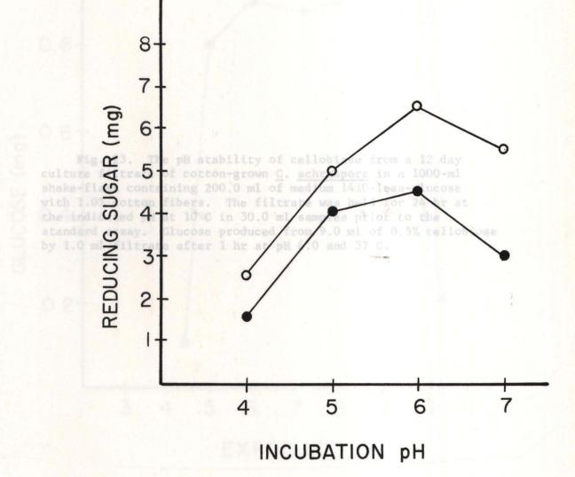
Fig. 23. The pH stability of cellobiase from a 12 day culture filtrate of cotton-grown <u>C</u>. <u>achraspora</u> in a 1000-ml shake-flask containing 200.0 ml of medium 1410-less-glucose with 1.0% cotton fibers. The filtrate was held for 24 hr at the indicated pH at 10 C in 30.0 ml samples prior to the standard assay. Glucose produced from 9.0 ml of 0.5% cellobiose by 1.0 ml filtrate after 1 hr at pH 6.0 and 37 C.
