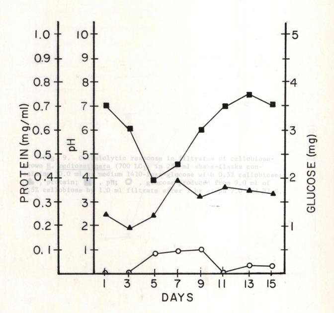
Fig. 9. Cellulolytic response in filtrates of cellobiosegrown <u>H. mediosetigera (700 LC<sub>1</sub>) in 250-ml shake-flasks containing 50.0 ml of medium 1410-less-glucose with 0.5% cellobiose: , protein; , pH; , glucose produced from 9.0 ml of 0.5% cellobiose by 1.0 ml filtrate after 1 hr at pH 7.0 and 37 C.</u>
