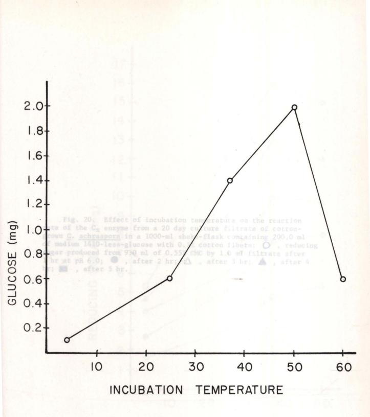
Fig. 20. Effect of incubation temperature on the reaction rate of the  $C_x$  enzyme from a 20 day culture filtrate of cottongrown <u>C</u>. <u>achraspora</u> in a 1000-ml shake-flask containing 200.0 ml of medium 1410-less-glucose with 0.5% cotton fibers:  $\bigcirc$ , reducing sugar produced from 9.0 ml of 0.55% CMC by 1.0 ml filtrate after 1 hr at pH 6.0;  $\bigcirc$ , after 2 hr;  $\triangle$ , after 3 hr;  $\blacktriangle$ , after 4 hr;  $\blacksquare$ , after 5 hr.
