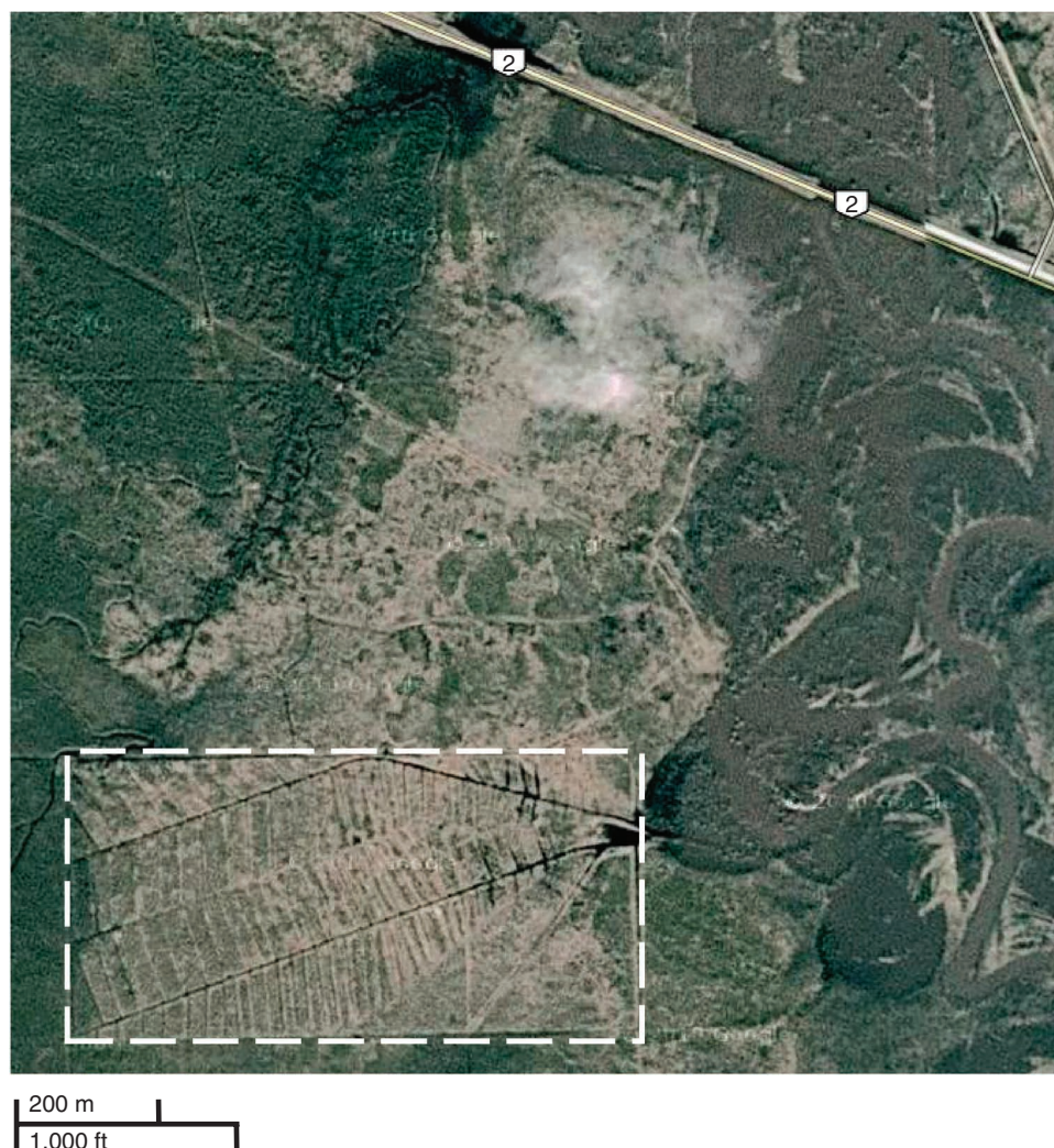
Figure 1 | Large-scale experimental drainage in a boreal fen. Aerial image of drainage trenches (outlined in dashed white line) in a boreal peatland in Alberta, Canada. ©2011 Google-Imagery ©2011DigitalGlobe, Cnes/Spot Image, GeoEye, Map data.
