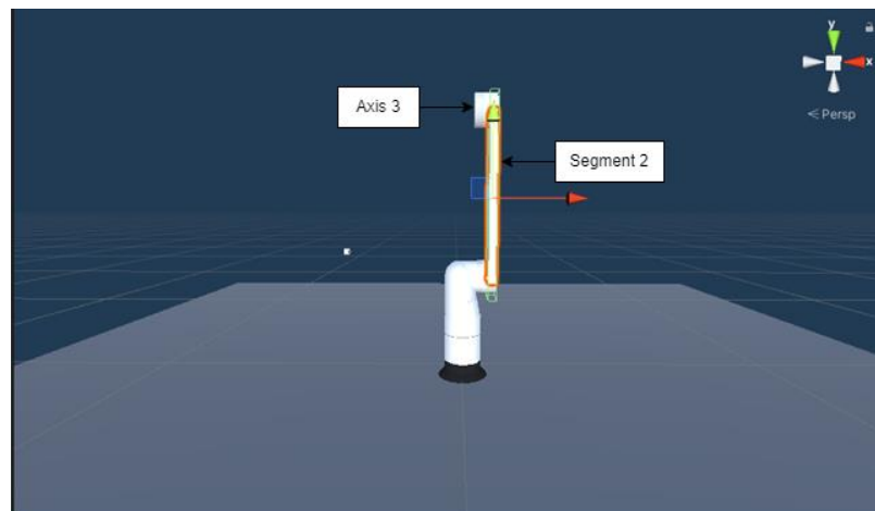
Figure 6 - Step 5 of creating the Kinova Robotic Arm model: create segment 2 of the arm and axis 3. Segment 2 is the long rectangle portion to the right of axis 2, and axis 3 is placed facing left at the top of segment 2.
