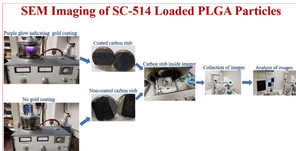
Figure 22. Schematic illustration of scanning electron microscopy (SEM) imaging of SC-514 loaded PLGA nanoparticles. The lyophilized nanoparticles were mounted on a carbon stub. Gold palladium was then used to coat the surface of the nanoparticles in order to enhance the structural characteristics of the SC-514 loaded PLGA nanoparticles. The control group, consisting of non-coated nanoparticles, were also utilized to compare the data analysis with the gold coated SC-514 loaded PLGA nanoparticles. The carbon stub was inserted into the imager to take pictures of the nanoparticles. The pictures were collected, organized and analyzed.
