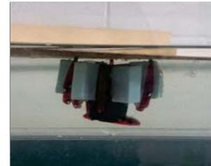
Illustration of inverted underwater walking capabilities
