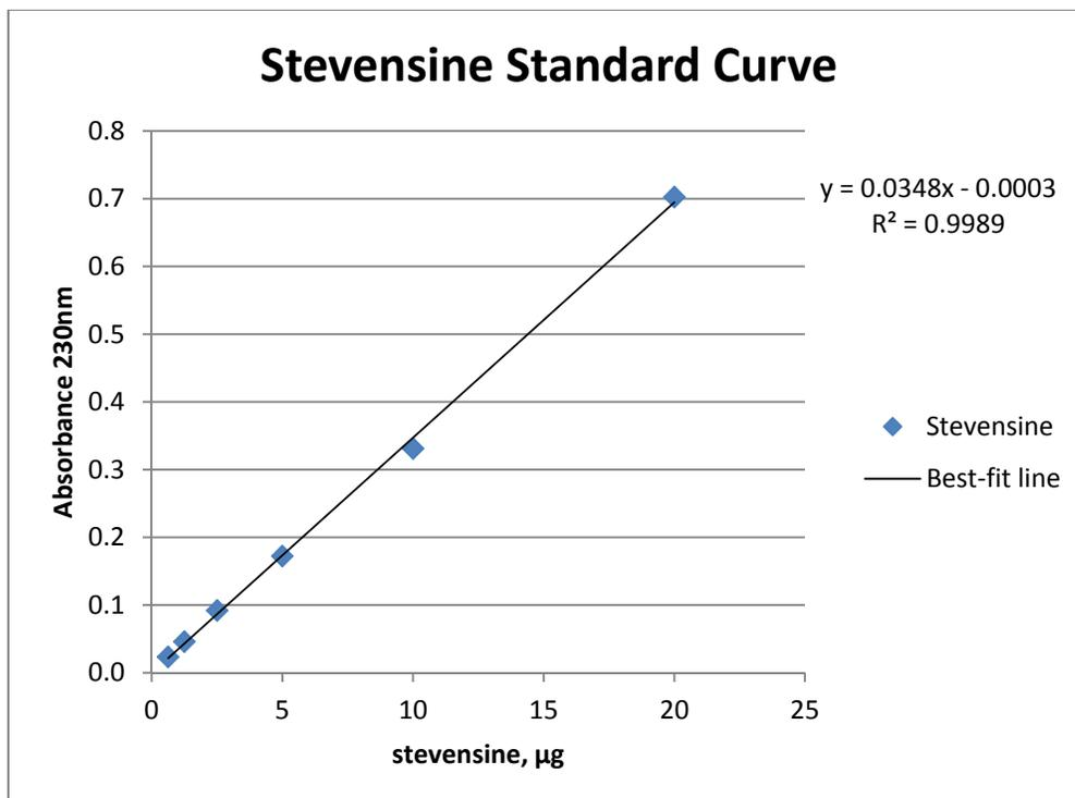
**Figure 4.** Serial dilutions of pure stevensine (31.25 – 1000 µg/ml) were used to derive a standard curve for quantification of test samples. Standard curve of pure stevensine analyzed at 230nm absorbance. Coefficient of determination = 0.9989.
