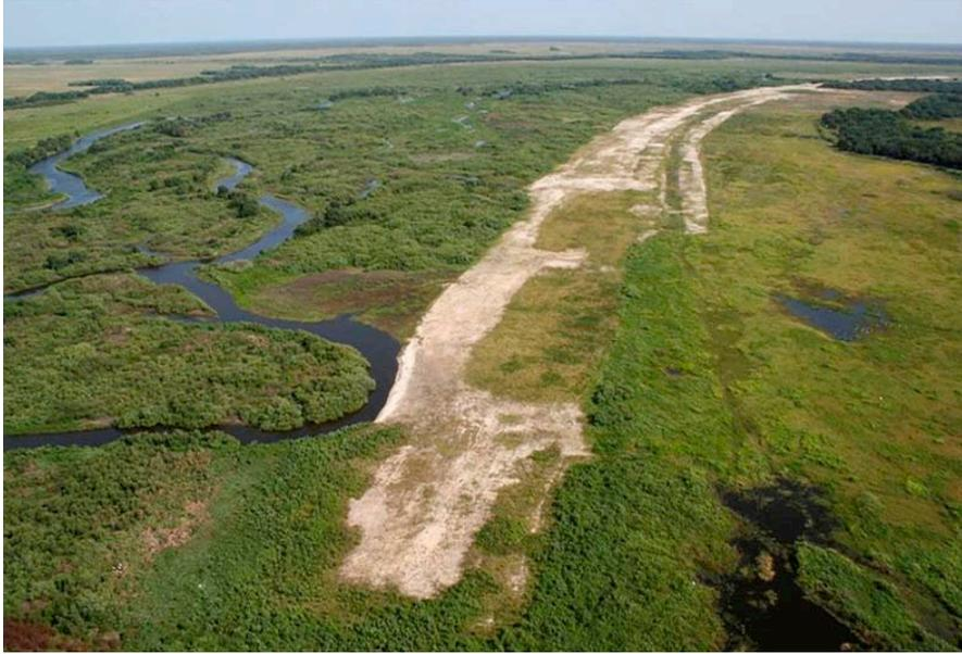
Figure 1: Photo of a section of the restored river with backfilled canal.
