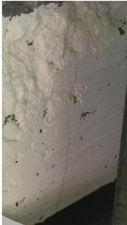
*Figure 4-2 First Crack in Specimen 1*
