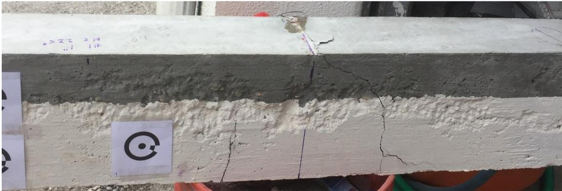
*Figure 4-3 Shear Flexure Cracking*
