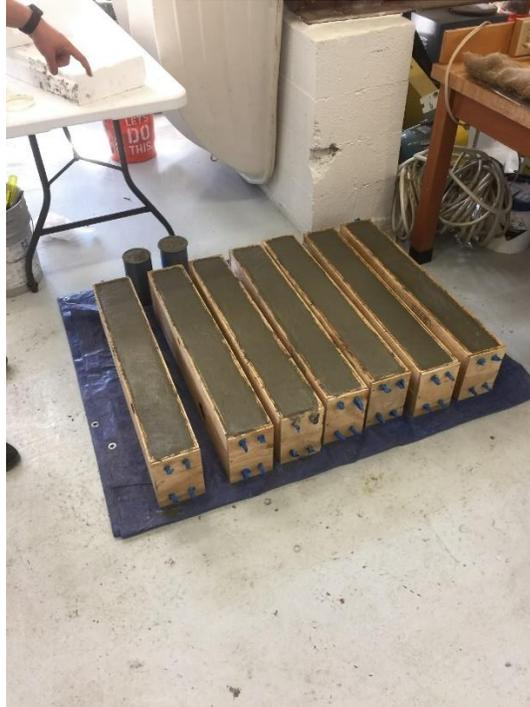
*Figure 3-4 Concrete Beams*
