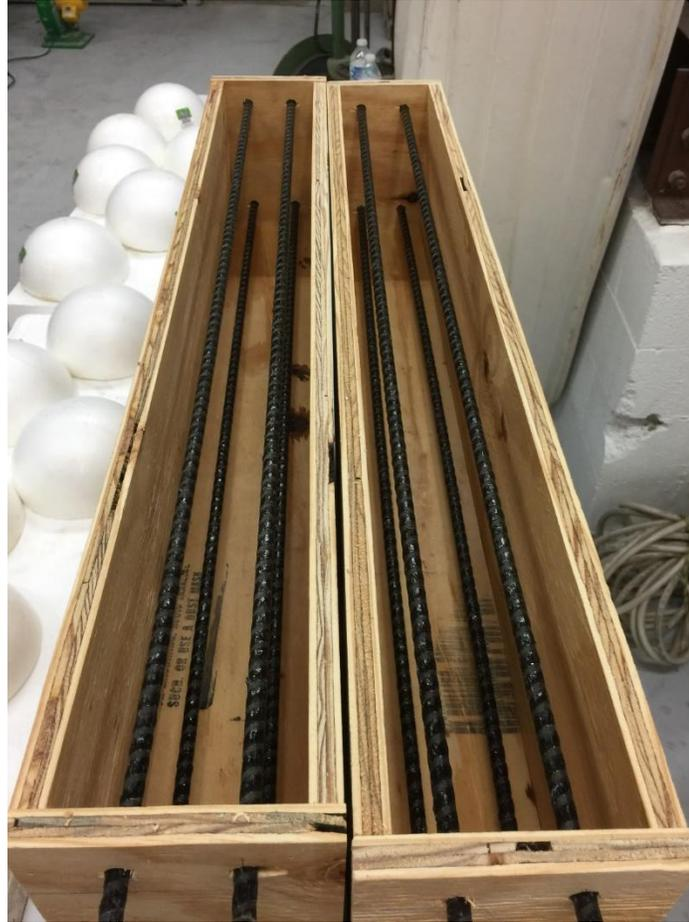
*Figure 3-3 BFRP Reinforcements Positioned in Plywood Forms*
