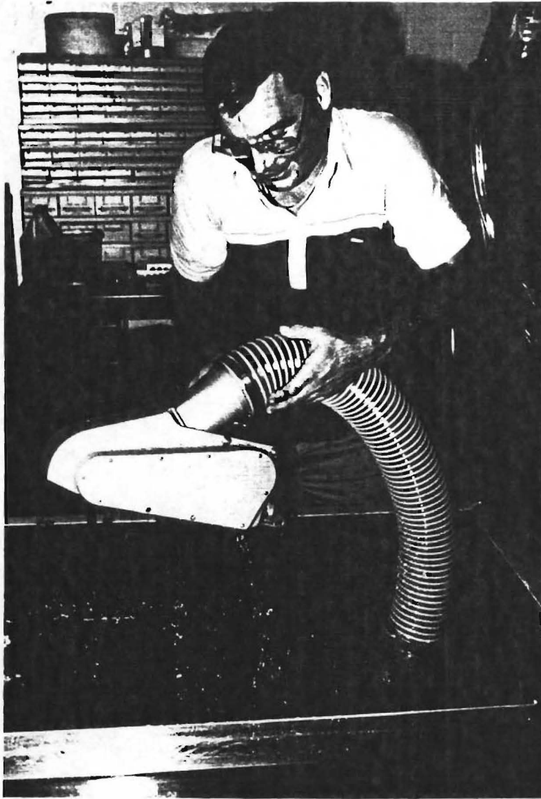
FIGURE 7. TANK TEST OF BRUSH SAMPLER
