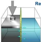
Reverse osmosis (or RO) is a process in which "water molecules are forced through a 0.0001 micron semi-permeable membrane by water pressure".<sup>2</sup> It is different
