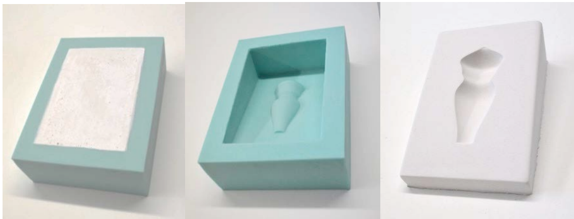
Figure 21. Rubber mold with the plaster piece
