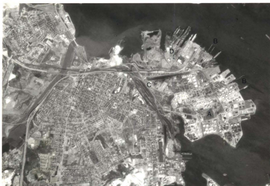
Figure 34. Petroleum storage tank field (A), narrow piers (B), railroad yard (C), shipbuilding yard (D).
