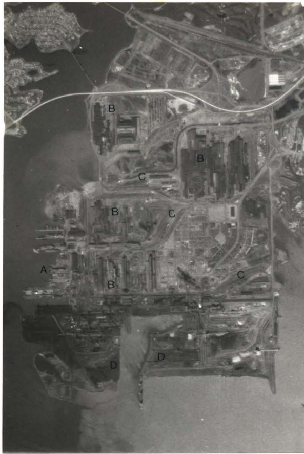
Figure 32. Shipbuilding (A) steel processing and fabrication (B), railroad (C), open storage (D). The shipbuilding yard (A) is also shown in Figure 33.
