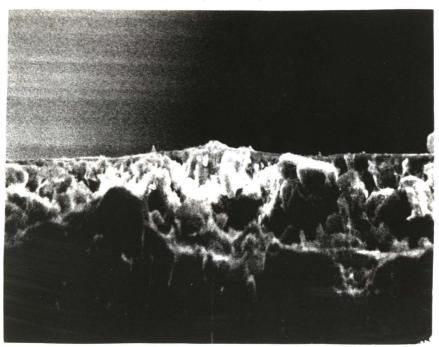
Figure 4-1 Photograph of Calcareous Deposits After Compression (#13 and #10, -0.85V SCE)
